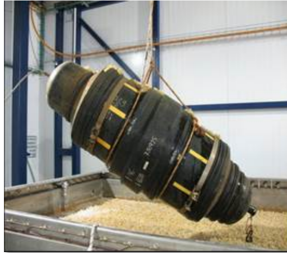
630 mm SDR17 gas pipe and EF coupler being lowered into hydrostatic bath
