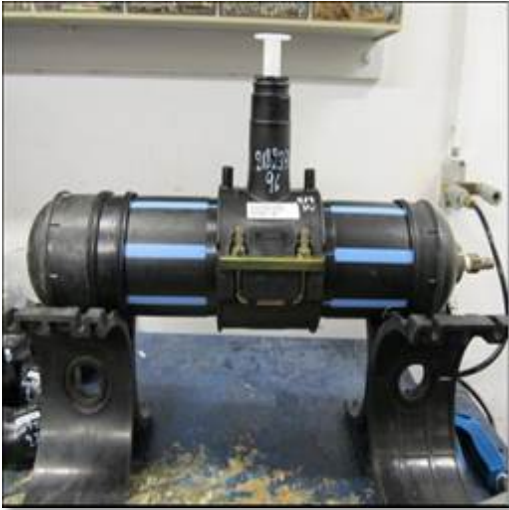
110 mm SDR17 water pipe and tapping saddle EF assembly ready for product testing
