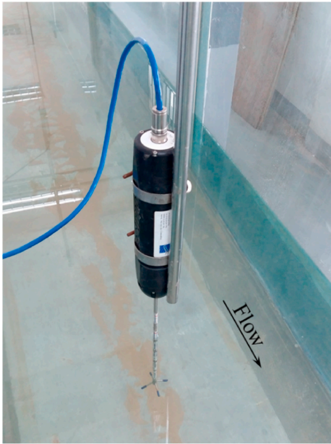
Fig. 5. (Color) Acoustic Doppler Velocimeter (ADV) used in the experiment. (For interpretation of the references to colour in this figure legend, the reader is referred to the Web version of this article.)
