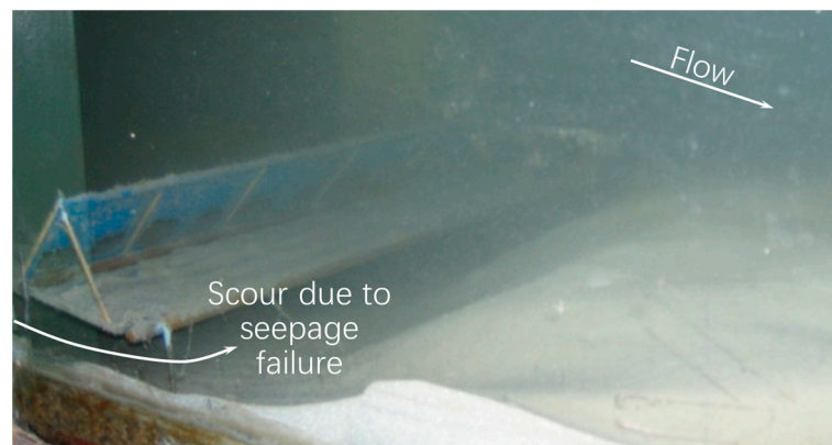
Figure 2. Scour beneath the mattress of a floating flow deflection structure [15].
