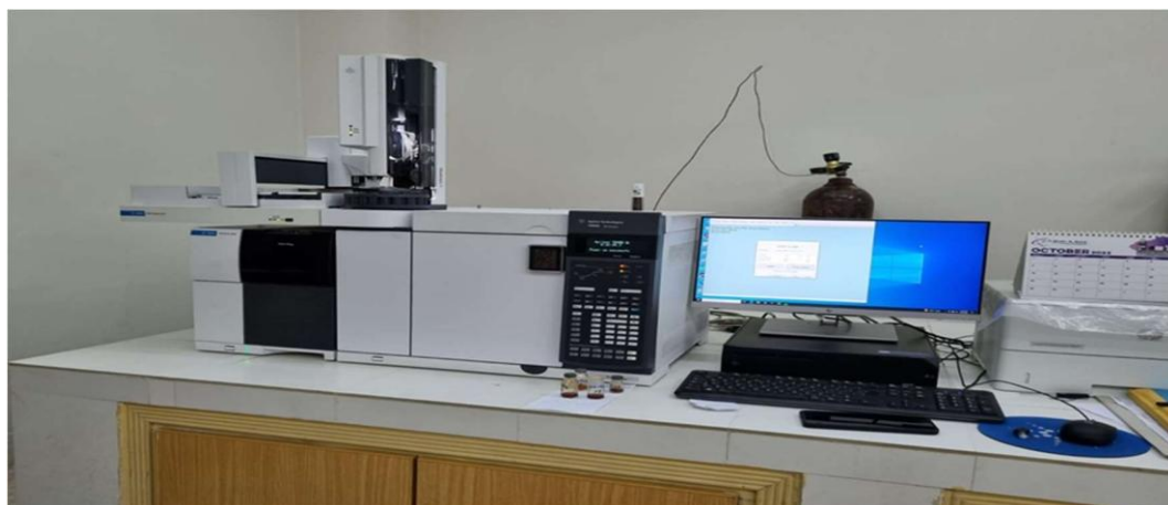
Figure 3 GC-MS used for qualification and quantification of chlorine DBPs
