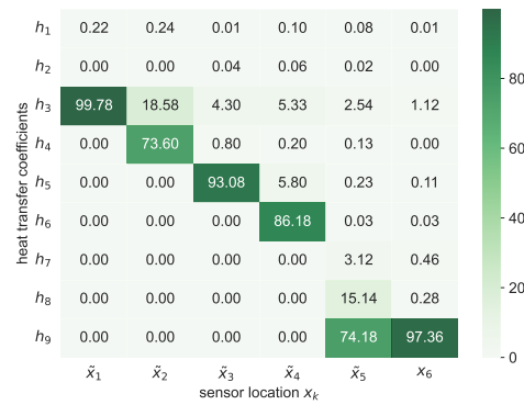
Figure 9: First order Sobol sensitivity indices for each unknown heat transfer coefficient h_i and sensor location ( \tilde{x}_k , x_k ).
