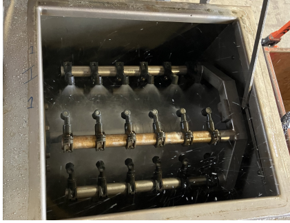
Figure 2: Active spray cooling in process step 1 as an example of forced convection with water as coolant.
