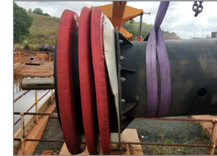
Figure 6: Damaged gauging plate
