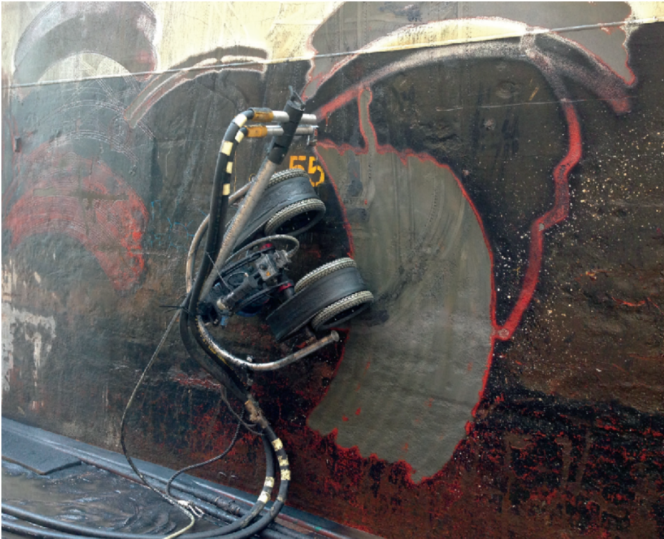
Fig. 2: This magnetically attached crawling unit performs grit-blasting on a ship's hull. Photos: Courtesy of Blastone International
