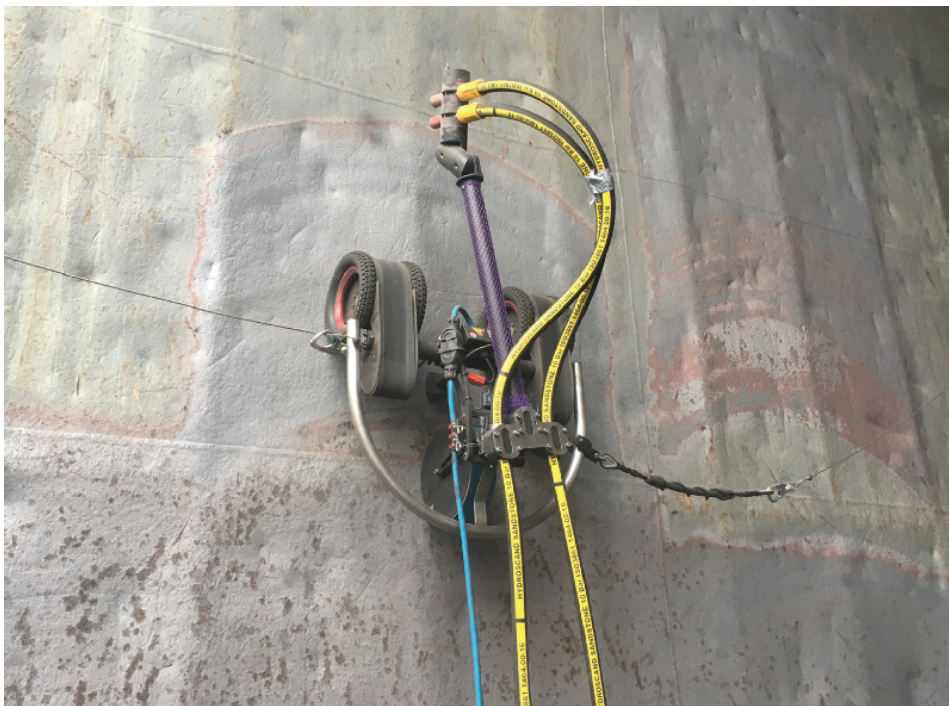
Fig. 1: Automated surface preparation units can be attached to ships' hulls for coating removal. Photo: Courtesy of Blastone International
