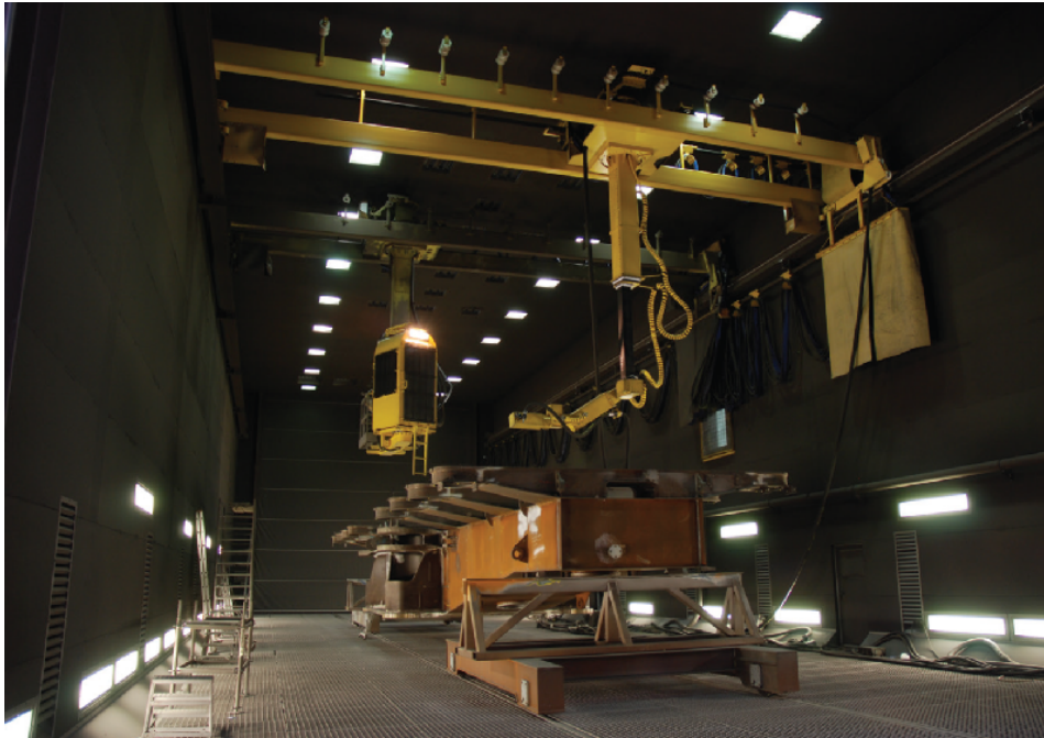
Fig. 5: Large robotic units can be used for thermal spray application, including the interior of pipes. Photo: Courtesy of Blastone International
