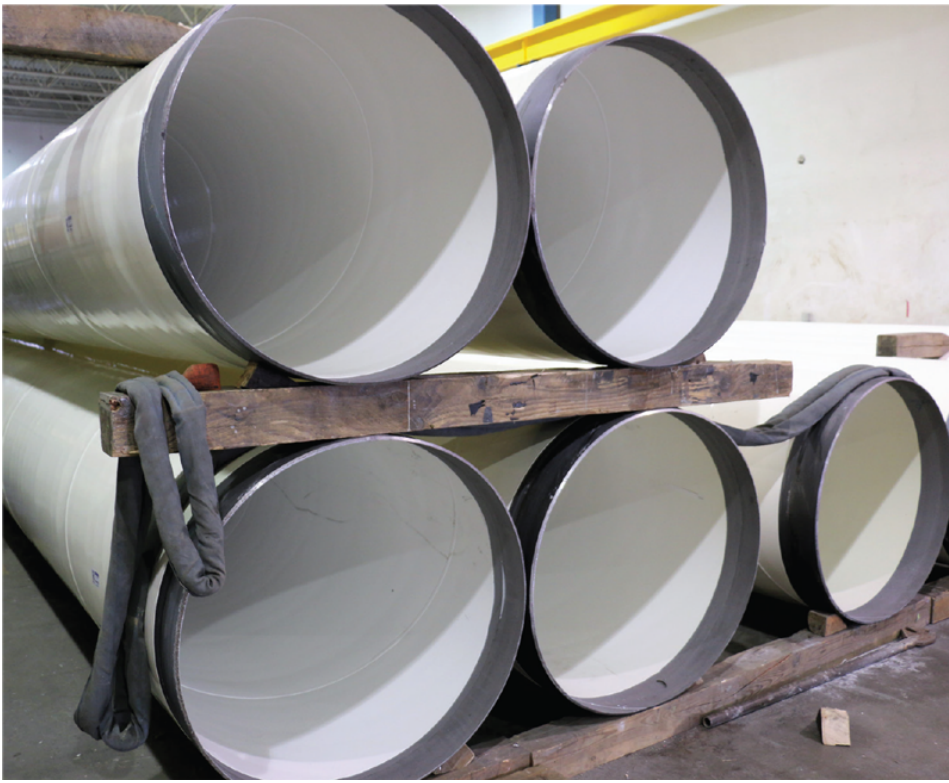
Fig. 4: The quick-set polyurethane exterior coating allowed the contractor to move completed pipes off its coating line and into staging areas for loading onto trucks in as little as 30–40 minutes, enabling timely deliveries to the pipeline installation site.
