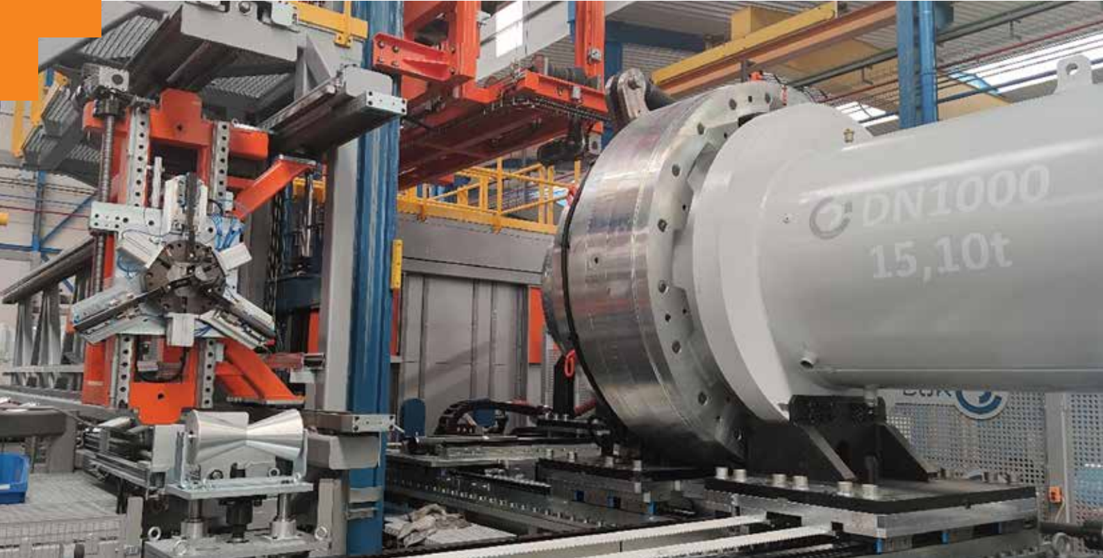
Molecor's DN 1 000 and M-OR-P 5012 mold under operation at the company's Madrid factory
