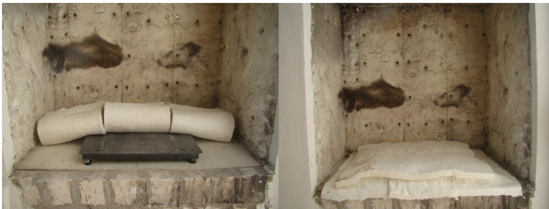
Figure 8. Industrial scales with a load of 600 kg protected with ceramic wool mattress
