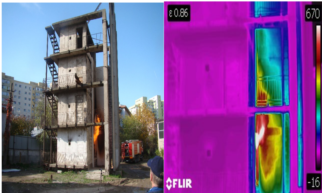
Figure 6. Images (photo and thermal) during flash-over
