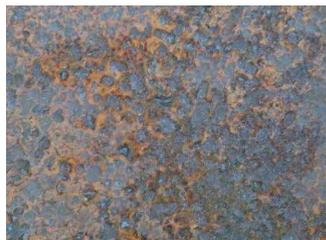
A corroded surface with pitting
