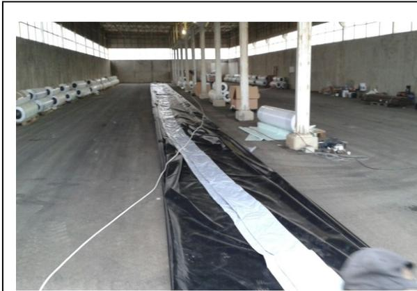
Figure 8. Local project facility plant for prefabrication of geomembrane panels (Genap, 2015)
