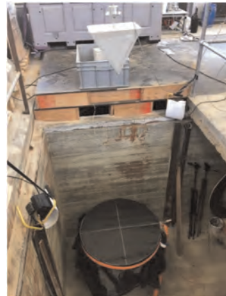
Figure 10. Drop tests with standardized stone shapes and weight on composite geotextiles (woven/non-woven) at Ghent University.
