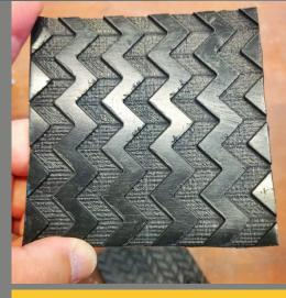
In a Laser Thermal Ablation (LTA) process, unwanted material is eliminated through the photo-thermal ablation effect. The patterns are "carved" into the top of smooth HDPE geomembranes. This process offers some big advantages such as:
