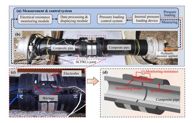
These smart strain-sensing EF fitting are made from HDPE compounded with Short Carbon Fibres (SCF) as shown in the process below. The network of interpenetrating carbon fibres can sense strain via a resistance measurement.
