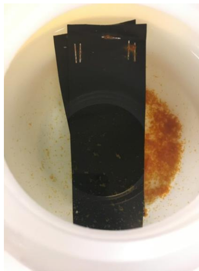
Figure 3. HDPE coupons in a combination of contaminated pond water with one of the flocculants at one week in the bath. Water has clarified by this time. Note floc at the bottom of the liquid from the applied chemical flocculant treatment. Also note the corrosion on the steel staples.
