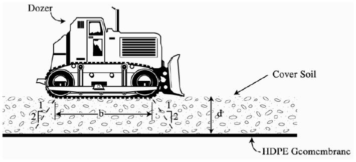
By far the most damage to a geomembrane is done during installation, particularly during covering (placement of the cover material). Stone punctures are the most frequent forms of damage with equipment damage the next. Relatively little new damage appears to occur during service. Thus protection systems have to be more effective during construction. The nature of the drainage layer over the geomembrane is critical.
