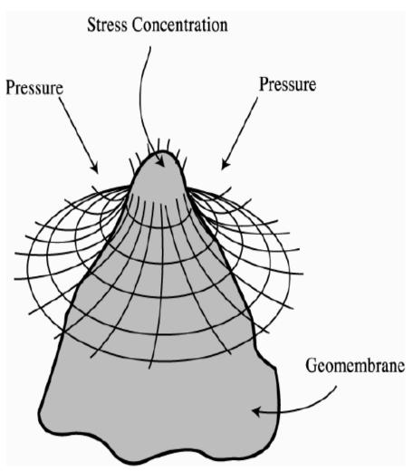
Damage is done to the geomembrane well before a leak/hole/puncture might occur in it. Therefore, damage can be done during installation that does not become a leak until later. Hence, the strict limitations on general (3%) and local (0.25%) strain imposed in Germany, and hence the thick/heavy geotextile and other protection systems.
