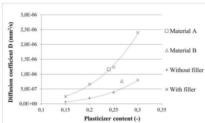
Figure 2. Results of plasticizer absorption tests at 75°C.
