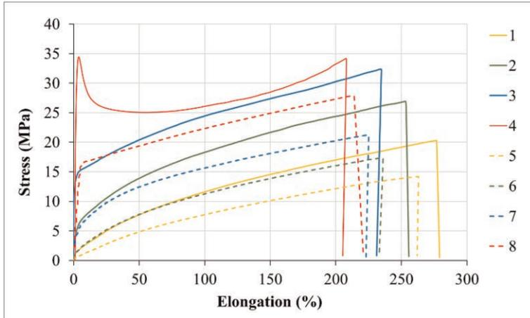
Figure 4. Tensile tests results on the 8 produced geomembranes.
