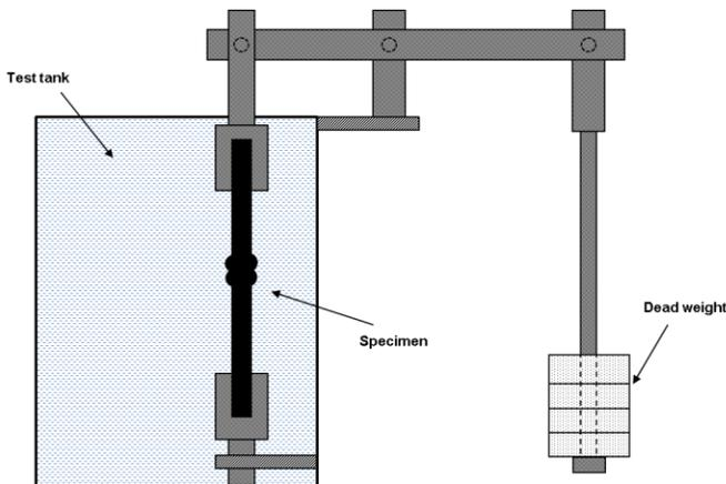
**FIG. 9 TENSILE CREEP RUPTURE TEST RIG, ACCORDING TO EN 12814-3**
