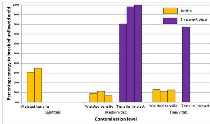
**FIG. 20 ENERGY TO BREAK WAISTED TENSILE TEST AND HIGH SPEED IMPACT TEST SPECIMENS FROM TALC-CONTAMINATED BUTT FUSION JOINTS IN 180MM SDR17 PE80 PIPE AS A PERCENTAGE OF ENERGY TO BREAK SPECIMENS FROM UNFLAWED JOINTS**
