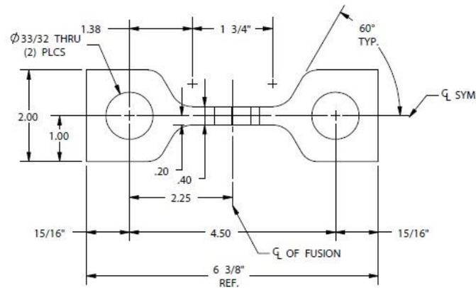
**FIG. 8 HIGH SPEED TENSILE IMPACT TEST SPECIMEN GEOMETRY, AS DEFINED IN ASTM F2634**
