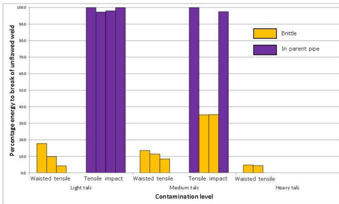
**FIG. 22 ENERGY TO BREAK WAISTED TENSILE TEST AND HIGH SPEED IMPACT TEST SPECIMENS FROM TALC-CONTAMINATED BUTT FUSION JOINTS IN 450MM SDR17 PE100 PIPE AS A PERCENTAGE OF ENERGY TO BREAK UNFLAWED JOINTS**
