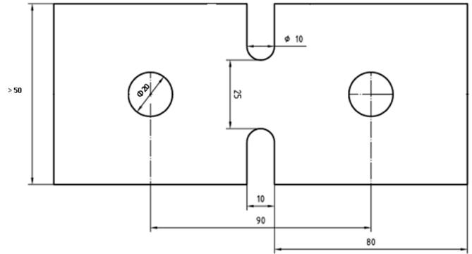
FIG. 6 TYPICAL GEOMETRY OF WAISTED TENSILE TEST SPECIMEN, AS DEFINED IN EN 12814-7
