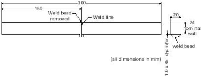
FIG. 3 TYPICAL GEOMETRY AND DIMENSIONS OF BEND TEST SPECIMEN, AS DEFINED IN EN 12814-1
