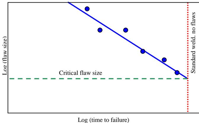
**FIG. 1 SCHEMATIC OF A GRAPH USED TO DETERMINE CRITICAL FLAW SIZES FOR LONG-TERM JOINT INTEGRITY**
