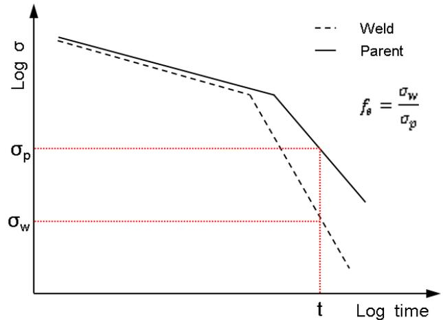
**FIG. 10 TYPICAL CURVES FOR THE COUPON CREEP RUPTURE TEST**
