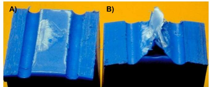
FIG. 7 EXAMPLE OF: A) BRITTLE FAILURE AND B) DUCTILE FAILURE IN A TENSILE TEST WITH A WAISTED SPECIMEN GEOMETRY
