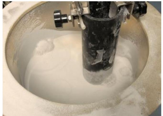
**FIG. 13 APPLICATION OF COARSE PARTICULATE CONTAMINATION ON TO THE END OF A PE PIPE USING A FLUIDIZED SAND BED**
