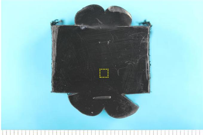
**FIG. 15 PARTICULATE-CONTAMINATED BUTT FUSION SPECIMEN FOR  $\mu$ CT ANALYSIS**
