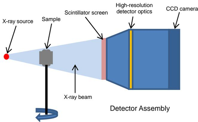
**FIG. 16 PRINCIPLE OF COMPUTED TOMOGRAPHY**
