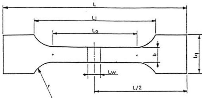
FIG. 5 TYPICAL GEOMETRY OF DUMB-BELL TENSILE TEST SPECIMEN, AS DEFINED IN EN 12814-2
