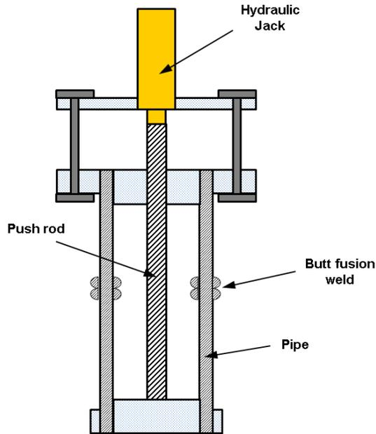
**FIG. 11 WHOLE PIPE TENSILE CREEP RUPTURE TEST, ACCORDING TO ANNEX B OF EN 12814-3**
