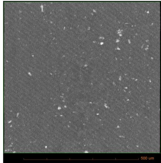
**FIG. 17 VIRTUAL SECTION THROUGH A  $\mu$ CT TOMOGRAPH OF A PARTICULATE-CONTAMINATED BUTT FUSION SPECIMEN**
