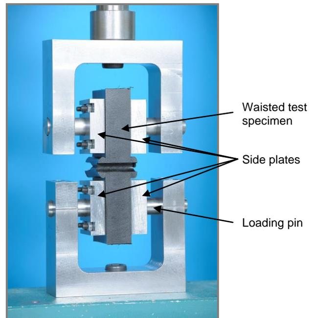
**FIG. 18 EXPERIMENTAL SET UP FOR TENSILE TEST WITH WAISTED SPECIMEN**
