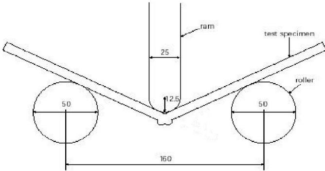
FIG. 4 SCHEMATIC DIAGRAM OF BEND TEST AS DEFINED IN EN 12814-1
