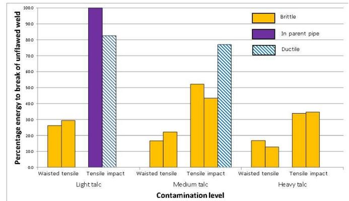
**FIG. 21 ENERGY TO BREAK WAISTED TENSILE TEST AND HIGH SPEED IMPACT TEST SPECIMENS FROM TALC-CONTAMINATED BUTT FUSION JOINTS IN 355MM SDR11 PE80 PIPE AS A PERCENTAGE OF ENERGY TO BREAK UNFLAWED JOINTS**
