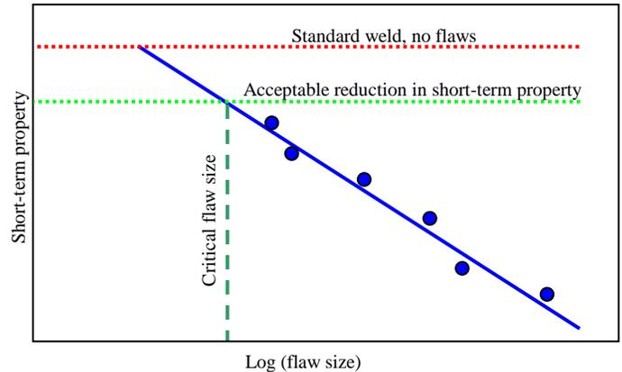
**FIG. 2 SCHEMATIC OF A GRAPH USED TO DETERMINE CRITICAL FLAW SIZES FOR SHORT-TERM JOINT INTEGRITY**
