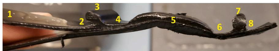
Fig. 3. Photo of the extrusion weld cross-section, which shows locations of the sampling for the Std-OIT test and crystallinity test.
