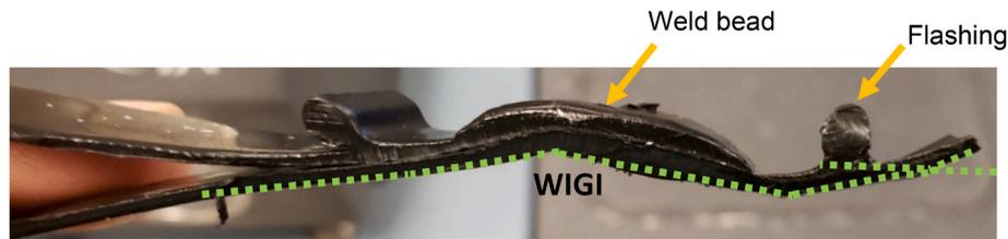
Fig. 2b. Photographic cross-section view of HDPE extrusion weld. (Welding induced geometric irregularity, WIGI).
