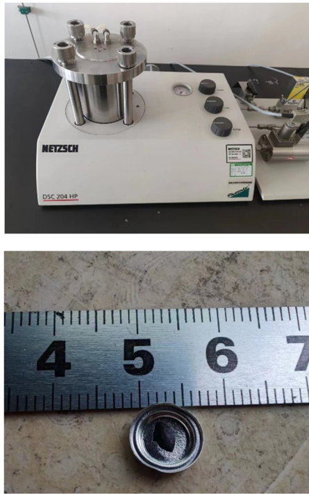
Fig. 3 NETZSCH 204 HP differential scanning calorimeter and test specimen
