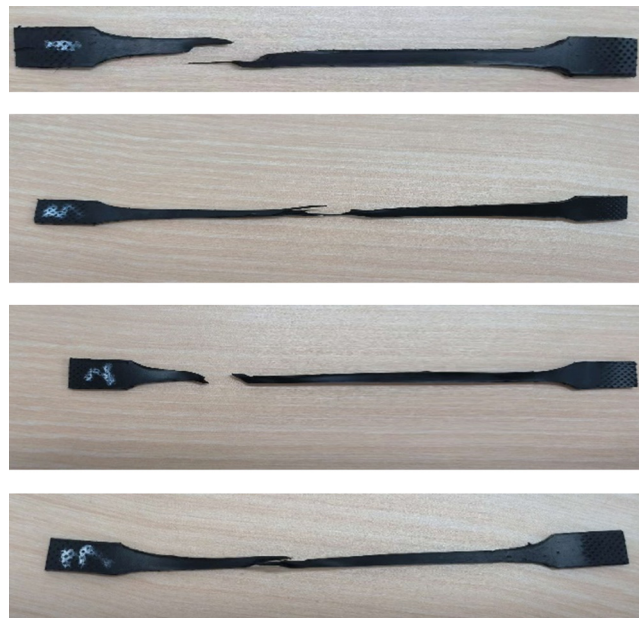
Fig. 6 Tensile test specimen under hydrostatic pressure (from up to down: test time 0 h, 200 h, 500 h, and 1000 h)
