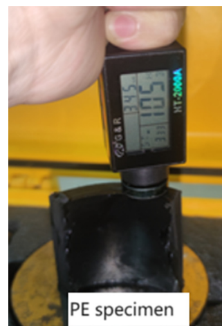
Fig. 2 Illustration of PE specimen hardness test
