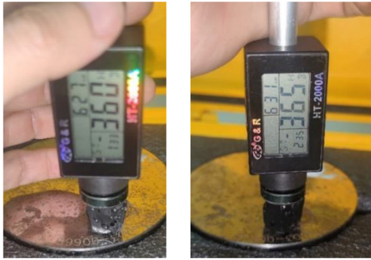
Artificial aging specimen
