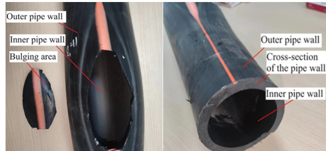
Fig. 16 DSC test samples location
