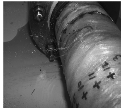
Fig. 5. (a) Variation of internal pressure for various winding angles with respect to time response (b) final fracture, and (c) leakage [94].
