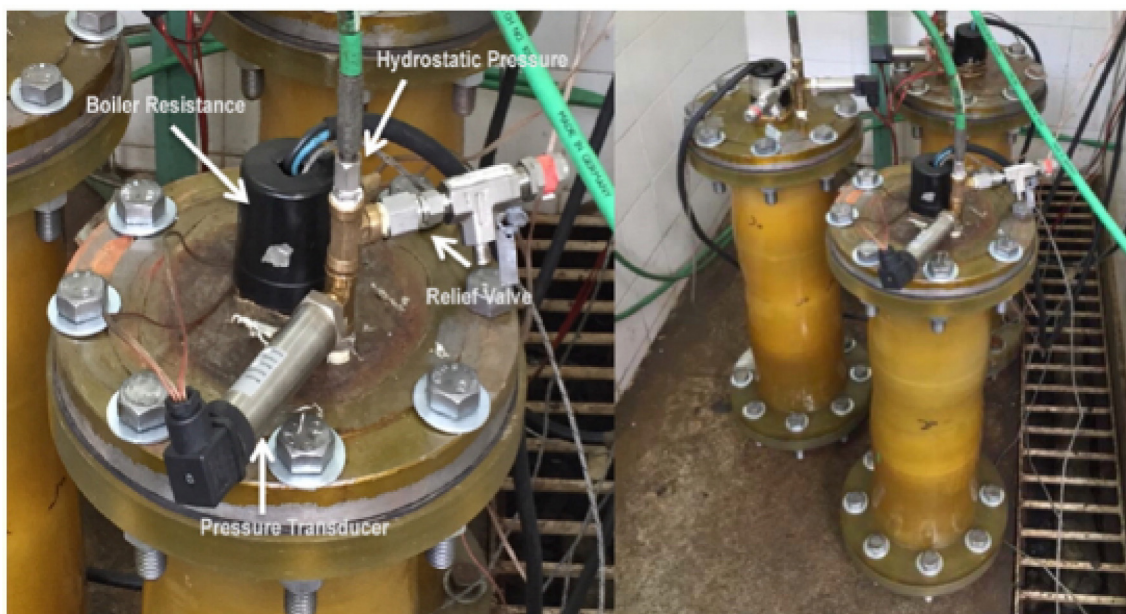
Fig. 12. Hydraulic test apparatus for prediction of burst failure pressure of FRP pipe under ageing conditions [165].
