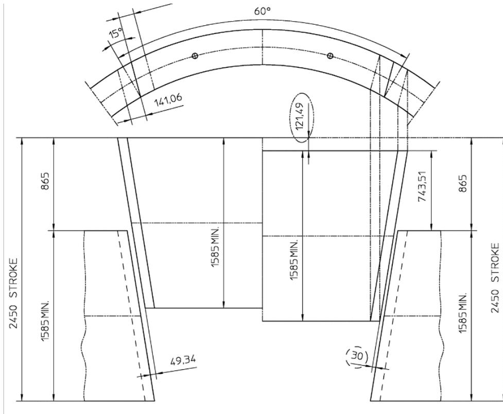
Figure 4. Key segment bevel geometry check to ensure constructability due to limitation on stroke length of TBM (source: Herrenknecht).
