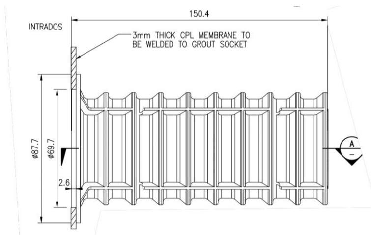
Figure 11. Detail of grout socket in main tunnel with HDPE lining welded directly to the grout socket.
