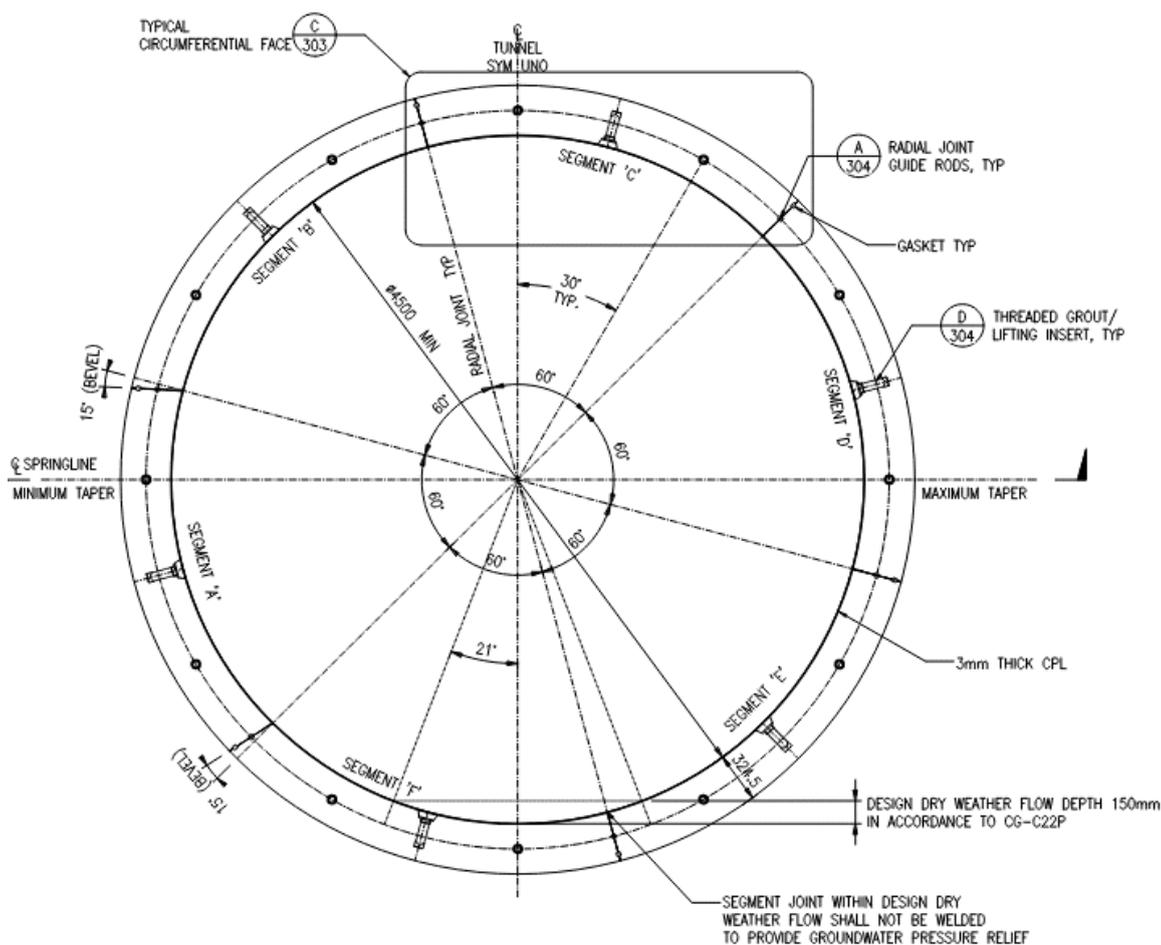
Figure 3. Cross section view of CI main tunnel.
