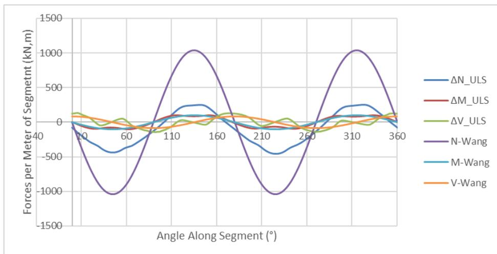
Figure 7. Comparison of seismic forces between FEA and no-slip condition by Wang (1993) at Shallow Tunnel Location in Soil (Residual ECBF)
