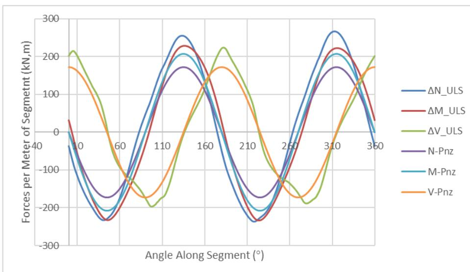
Figure 6. Comparison of seismic forces between FEA and no-slip analytical solution by Penzien (2000) at shallow tunnel location in soil (Tauranga Formation).
