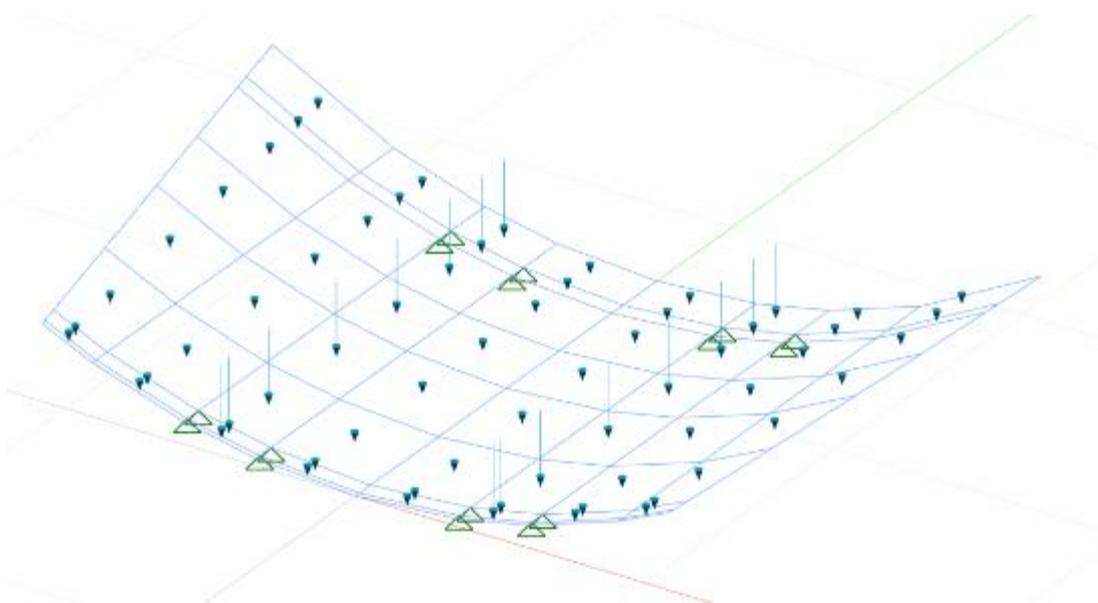
Figure 8. Sample structural model used to analyse the temporary loading condition of the segments.
