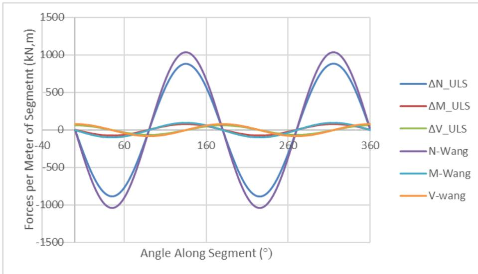
Figure 5. Comparison of seismic forces between FEA and no-slip analytical solution by Wang (1993) at deepest tunnel location in rock.
