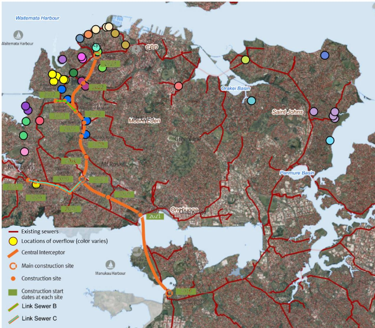
Figure 1. Central Interceptor alignment with existing wastewater network and current significant overflow locations (Watercare, 2016).
