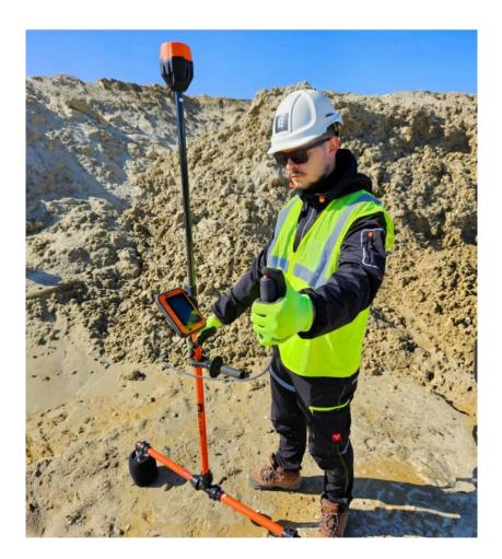
• The **eRover** takes automation to the next level, achieving survey speeds of 20,000 m<sup>2</sup> in eight hours and operating at depths of up to 1 meter.
