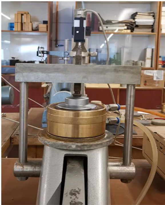
Figure 5. Oedometer cell specialized for falling head permeability test.
