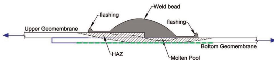
Figure 1. Cross-section of typical HDPE extrusion weld.
