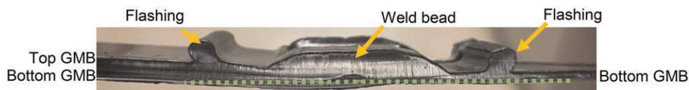
Figure 2. Photographic cross-section view of HDPE extrusion weld.
