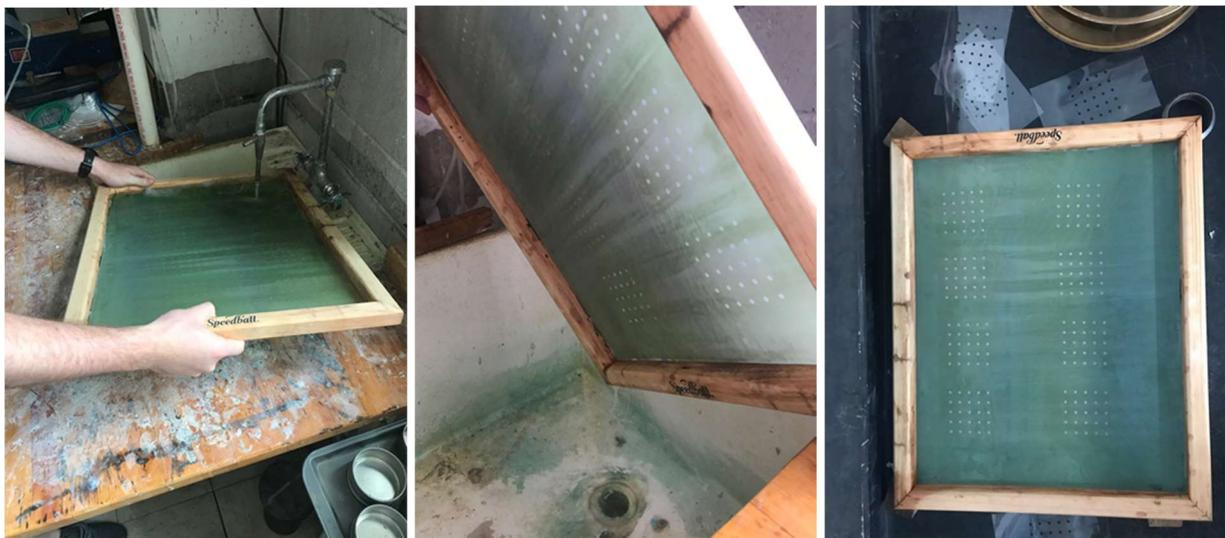
**Figure 2.7 Screen washing after light exposure.**
