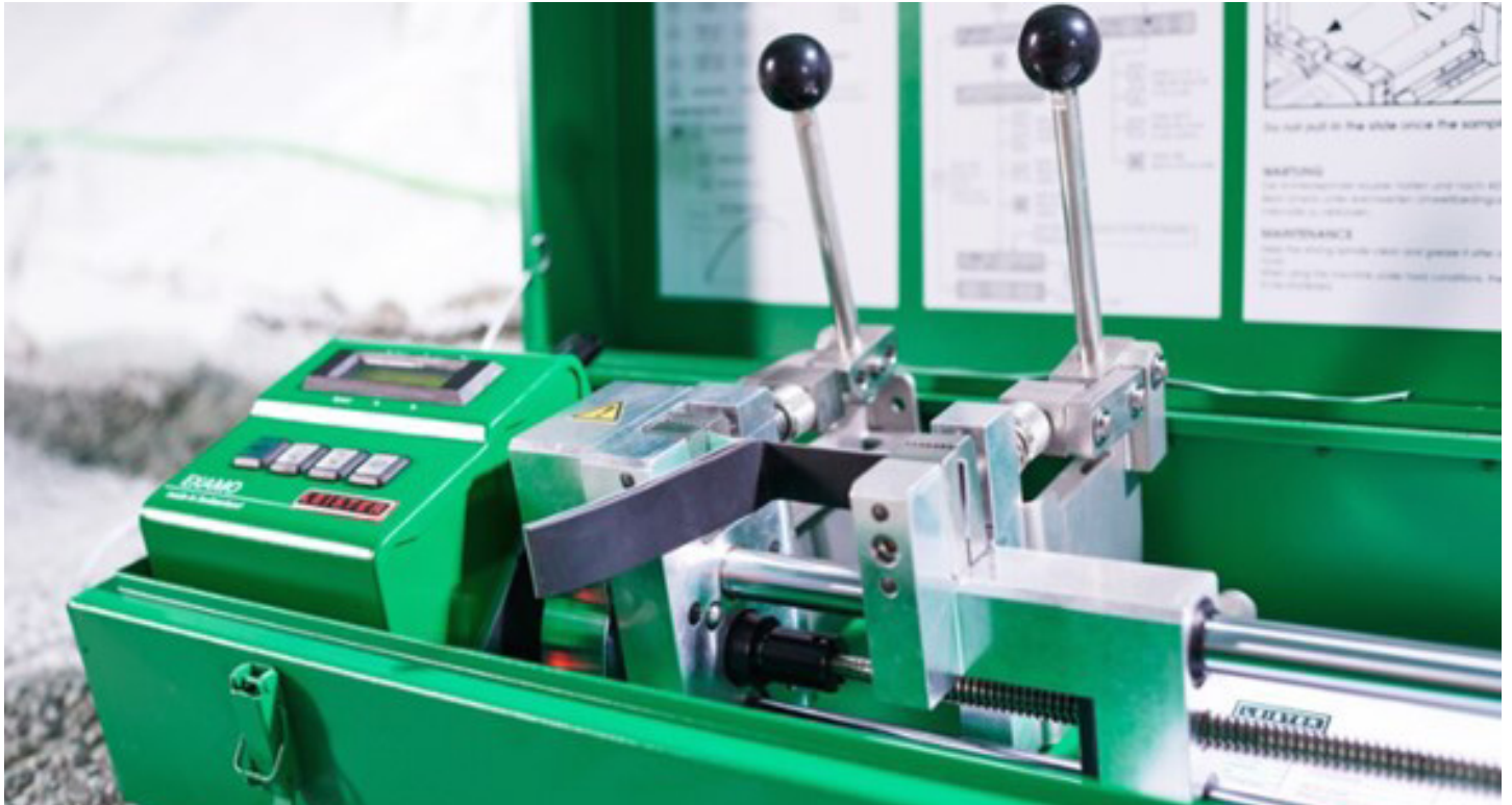
Figure 3: Examo tensiometer by Leister for CQA checks of weld strength. It is preferable that weld strength achieved is no less than 80% of the tensile stress of the BGM.
