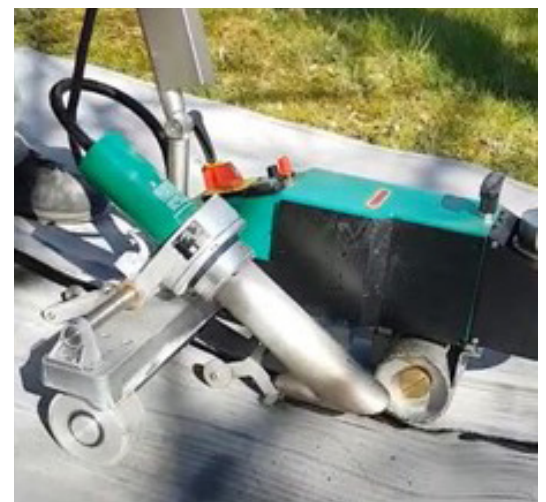
Figure 1: Bitumat B2 Leister in action with Teranap TP631. Testing was done over grass to simulate a rough surface during a typical installation.
