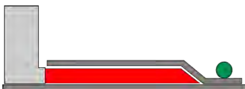
▲ Profile of hot air welding schematic featuring the hot air nozzle in red and air dam in green.
