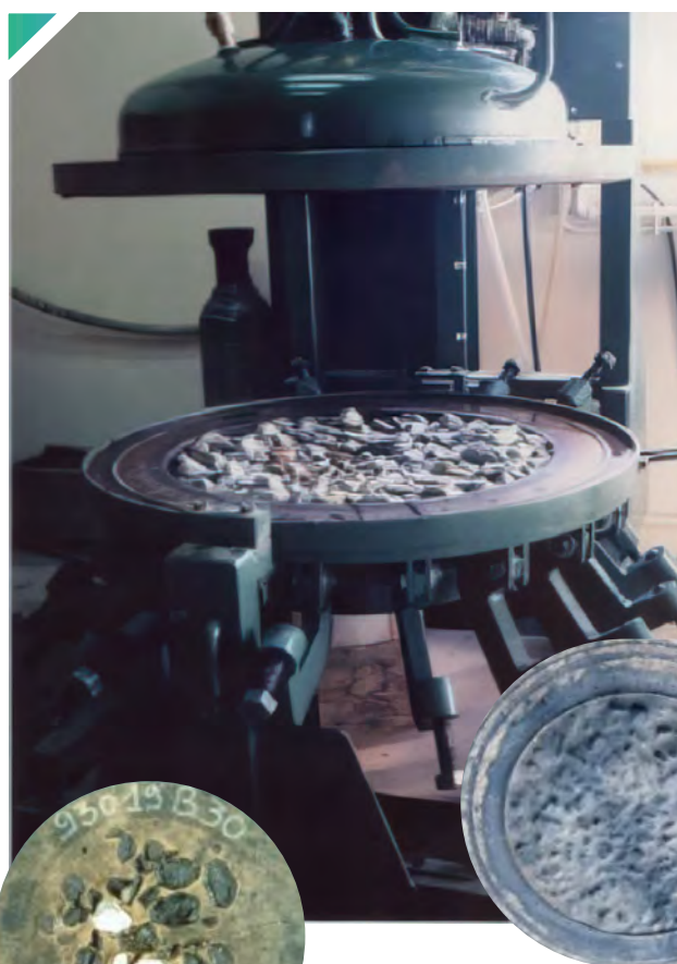
▲ Pu- ncture by aggregates results: no holes
