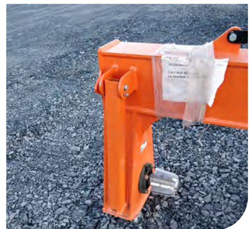
▲ Mandrel mounting point on the Hydraulic Beam
