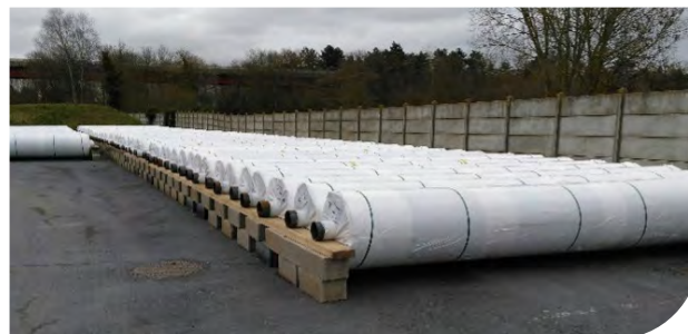
▲ Storage using concrete blocks and wooden beams
