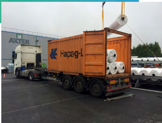
▲ Unloading using a spreader bar from a special open top container.
