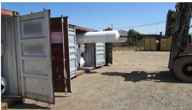
▲ Slightly lift the roll: the full weight of the roll should only be on the pin once it is fully inserted into the mandrel
