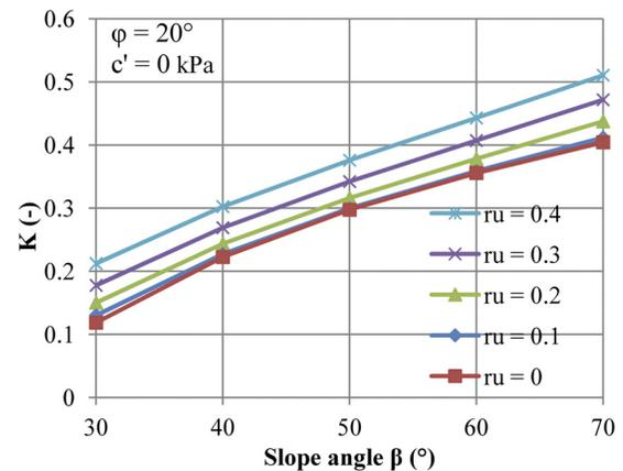
**Fig. 4.** Effect of pore-water pressure ratio  $r_u$  on the required strength of reinforcement (expressed by  $K$ )
