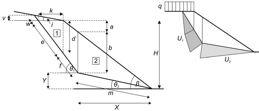
**Fig. 2.** Definition of two-part wedge geometry and total water pressures acting on the boundaries of each wedge
