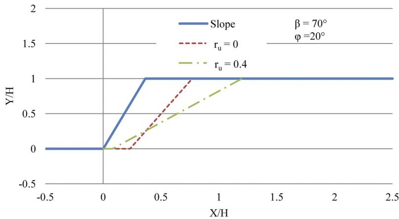
Fig. 5. Critical failure surface for various pore-water pressure ratios
