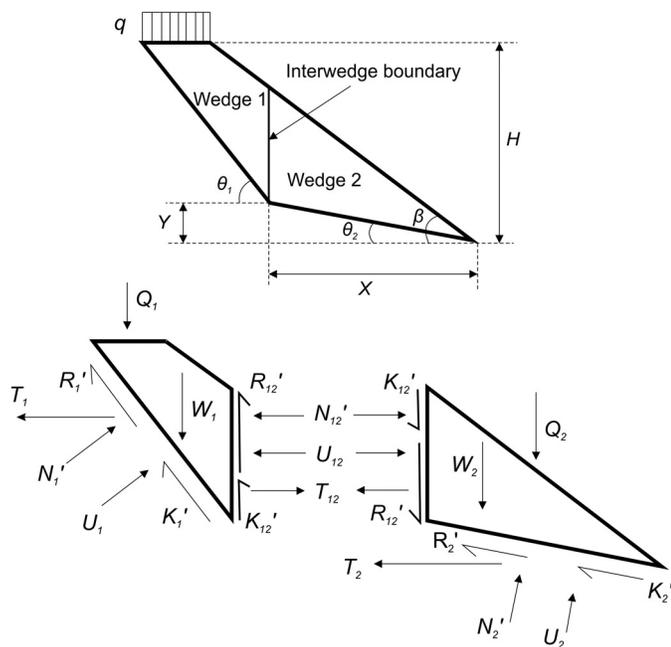
Fig. 1. Two-part wedge failure mechanism
