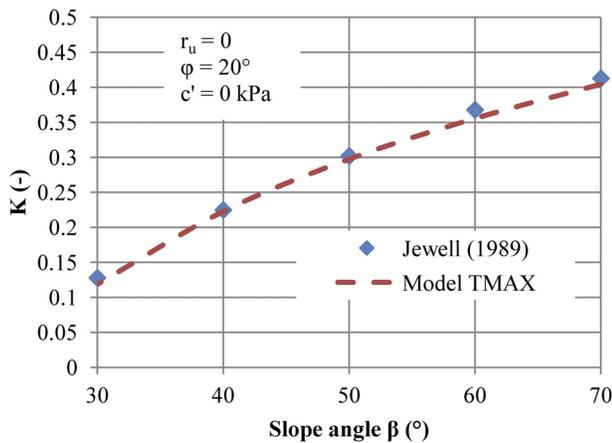
**Fig. 3.** Comparison of the required strength of reinforcement (expressed by  $K$ ), obtained using the TMAX model and the log spiral failure mechanism
