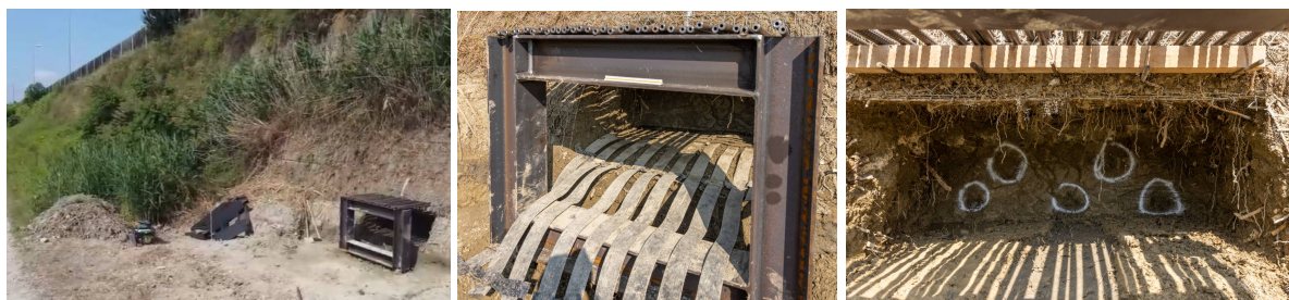
Figure 2. Exhumation of geogrids (550 kN/m and 150 kN/m) in Forlì and collection of the soil samples.
