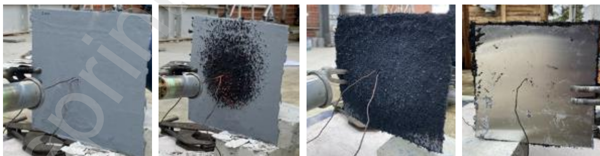
(a) Before testing (b) Initially char formation (c) Fully char formed (d) Unexposed side after testing
