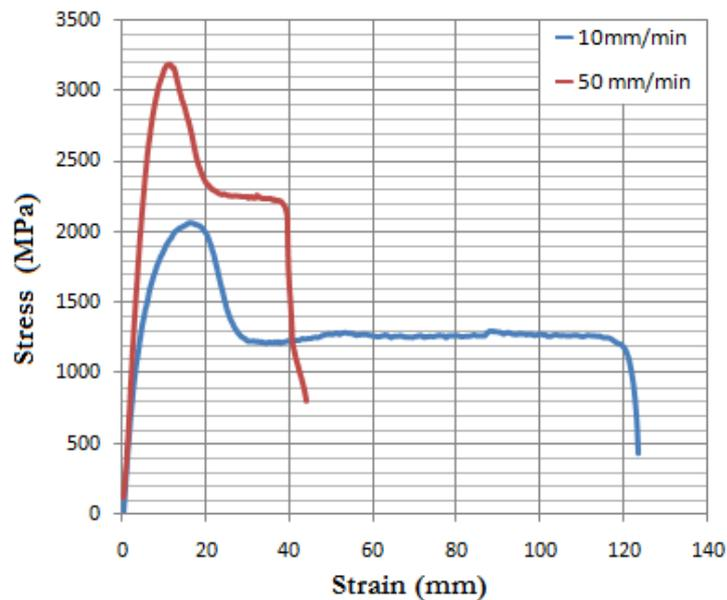
**Fig. 5.** Stress-Strain curve of test pieces without cracking
