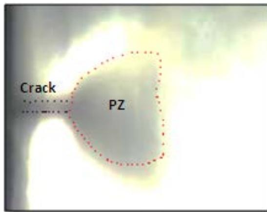
**Fig. 4.** Plastic zone (ZP) illustration at the crack end
