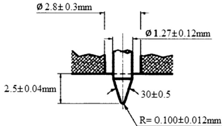
**Fig. 3.** Hardness shore D indentation and measurement
