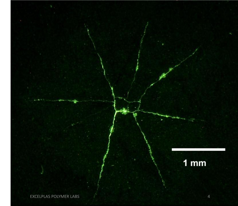
The new method using a fluorescent tracer to highlight the cracks in polymers under a UV microscope enabling greater sensitivity and contract enhancement
