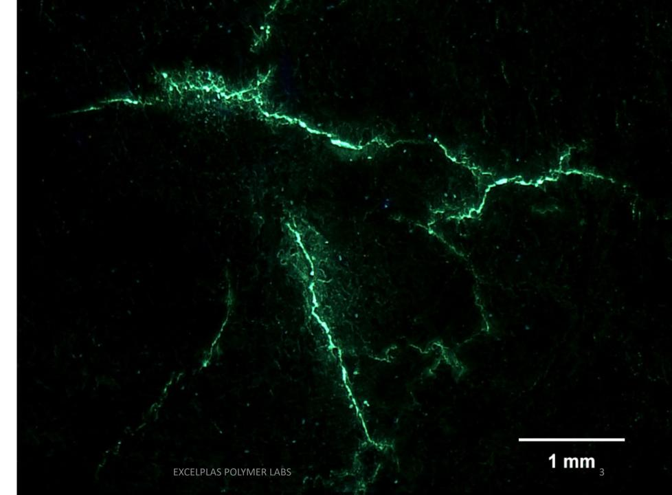
The new method using a fluorescent tracer to highlight the cracks in polymers under a UV microscope enabling greater sensitivity and contract enhancement
