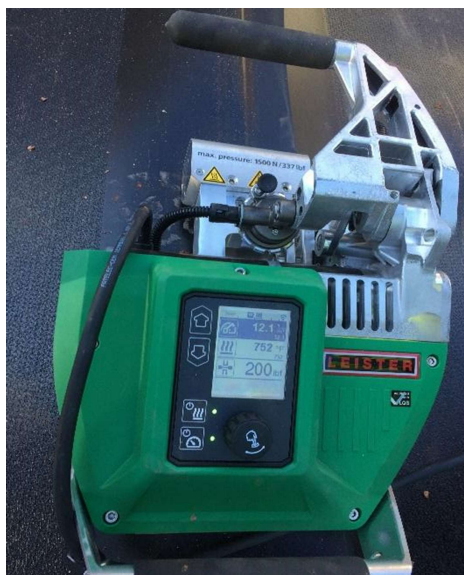
Figure 4: Data Acquisition Welding machine with visual display showing speed, temperature, and pressure.
