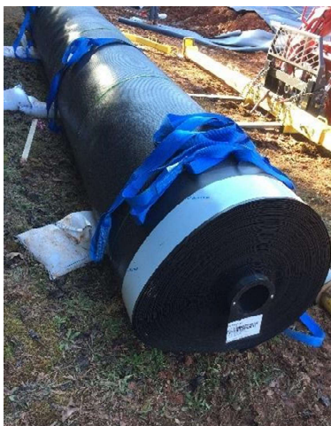
Figure 2: Geomembrane with taped edge.
