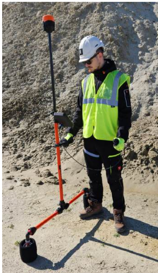
RTK GPS eDipole survey probe with display, RTK GPS unit and a trigger for easy data collection
