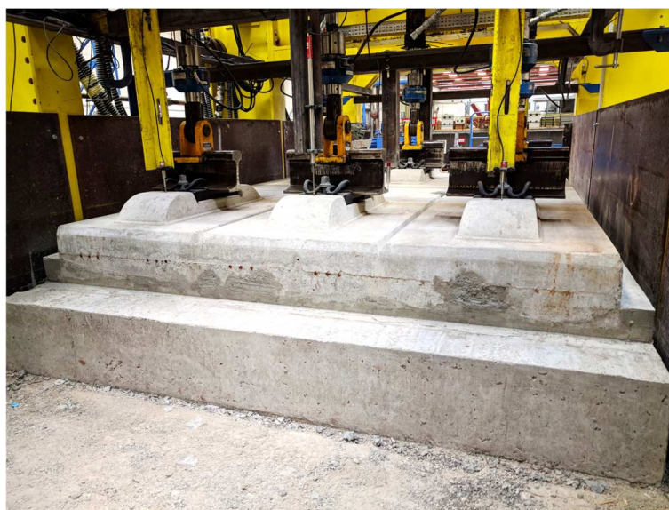
Figure 5. Slab track in the GRAFT-II testing facility.
