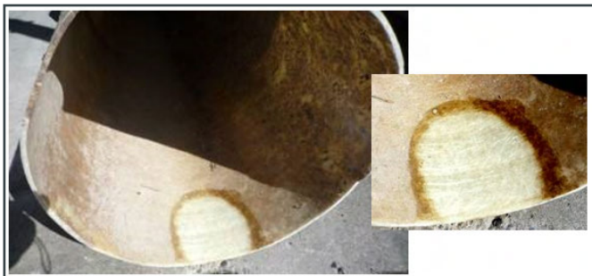
Figure 7: Flowtite pipe sample taken out from service after 30 years of operation.
