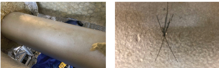
Fig. 11: At left is a photo taken during inspection of the hot-spread epoxy phenolic coating after seven months in service. The right exhibits the X-cut adhesion test, showing a rating of 10.
