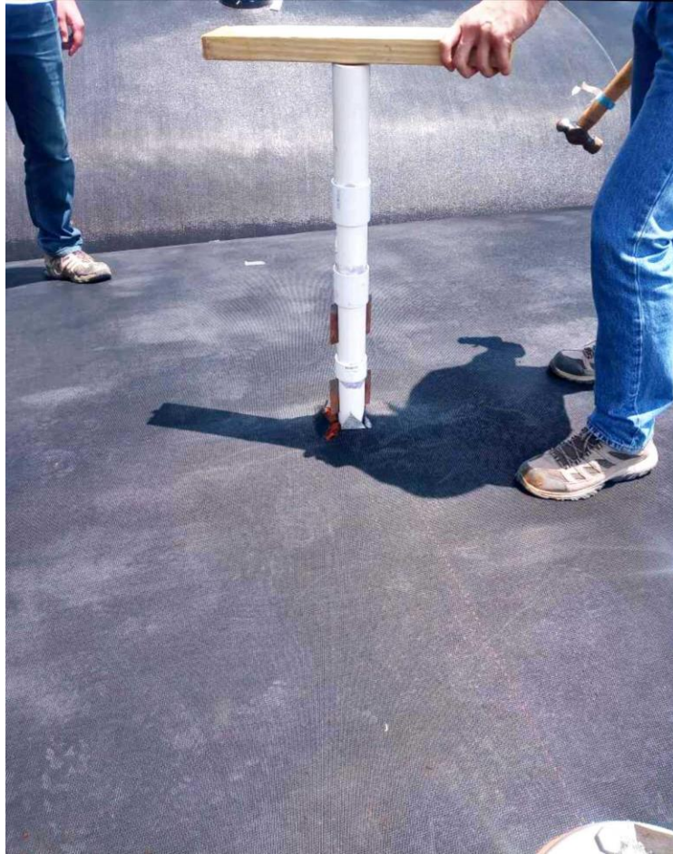
Figure 12: Moisture Distribution Sampler with 2x4 board (Source: Tyson 2022)
