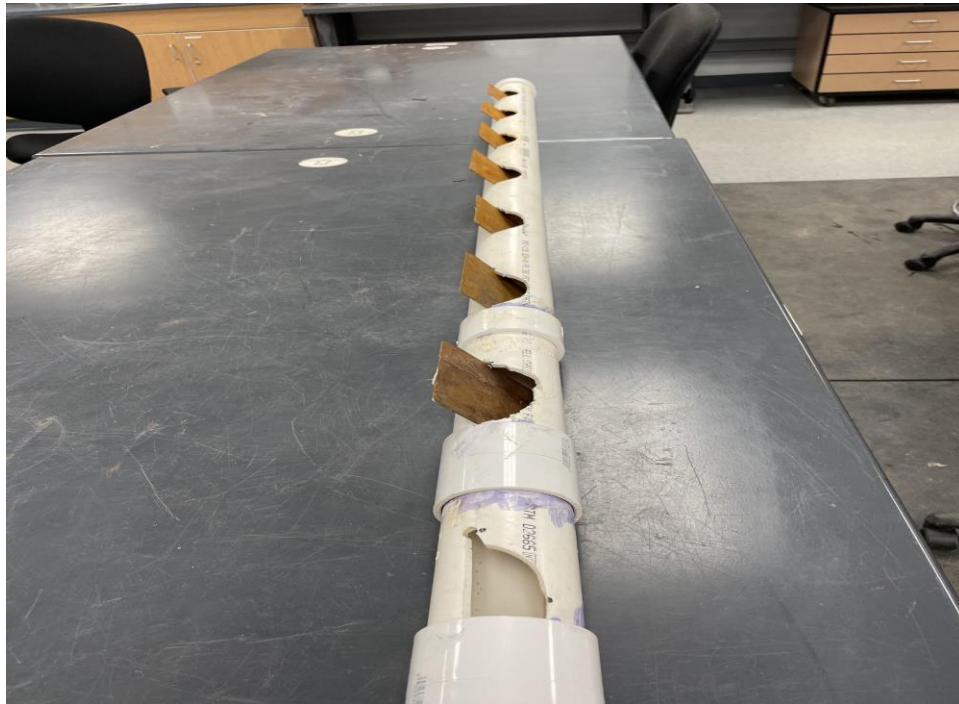
Figure 11: Version 2 6ft Sampler with 7 holes (Source: Tyson 2022)
