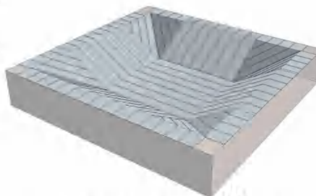
Diagram of cement blanket laying for reservoir
