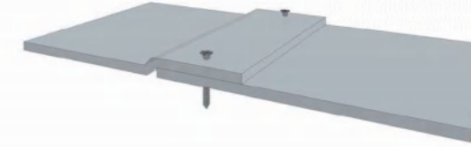
Method 1: Screw lap joint
