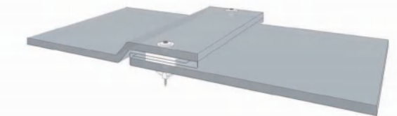
Method 6: customized lap joint
