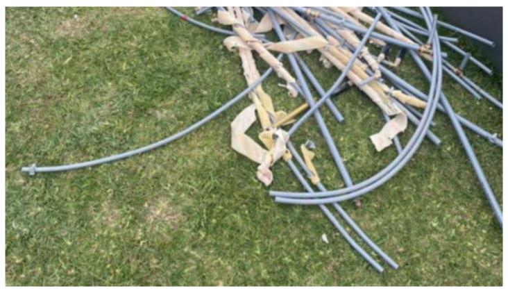
Defective polybutylene plumbing pipes have been stripped out of hundreds of new homes in WA. Credit: Unknown/Supplied
