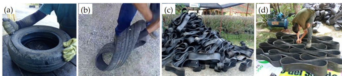
Figure 1. Manufacturing process of geocells made from recycled tires. (a) Sidewall cutting, (b) tread flipping, (c) assembly of the eights, (d) joining of the eights.
