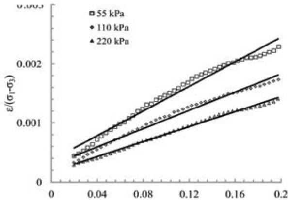
Fig. 5 : Plot between axial strain/deviator stress versus axial strain for pure clay
