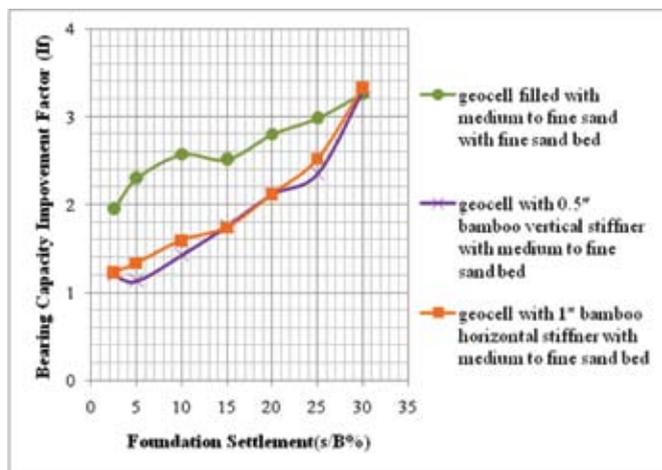
Fig. 8 : Bearing Capacity Improvement factor for Test series E and F
