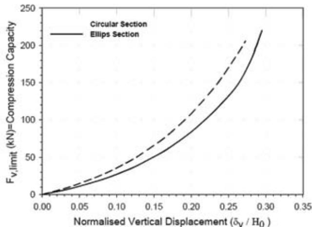
**Fig. 4 :** Load-normalized vertical displacement diagram of soilbag
