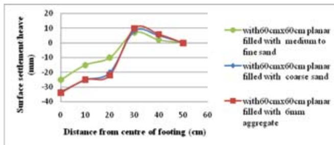
Fig. 10 : Heaving or settlement of clay surface for test series B
