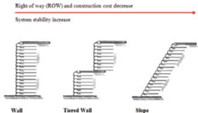
Fig. 1 : GRS structures with various configurations.
