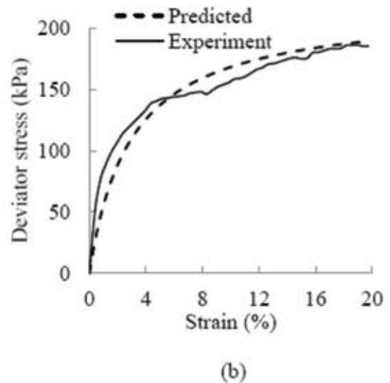
Fig. 10 : Predicted stress strain curves from hyperbolic model for clay reinforced with 0.25% untreated fibres with confining pressure of (a) 55 kPa and (b) 220 kPa
