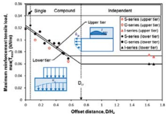
Fig. 4 : Effect of offset distance on maximum reinforcement tensile load
