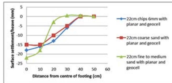
Fig. 12 : Heaving or settlement of clay surface for test series D
