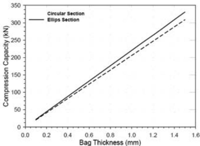
**Fig. 6 :** Variation of compression capacity with bag thickness
