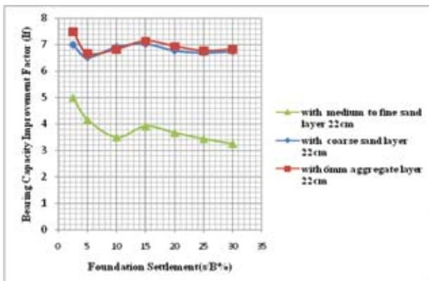
**Fig. 4** : Bearing Capacity Improvement factor with respect to clay bed for Test series A
