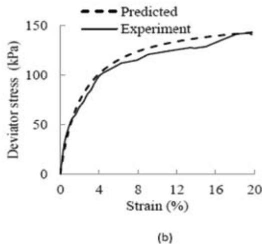
Fig. 9 : Predicted stress strain curves from hyperbolic model for clay with confining pressure of (a) 55 kPa and (b) 220 kPa
