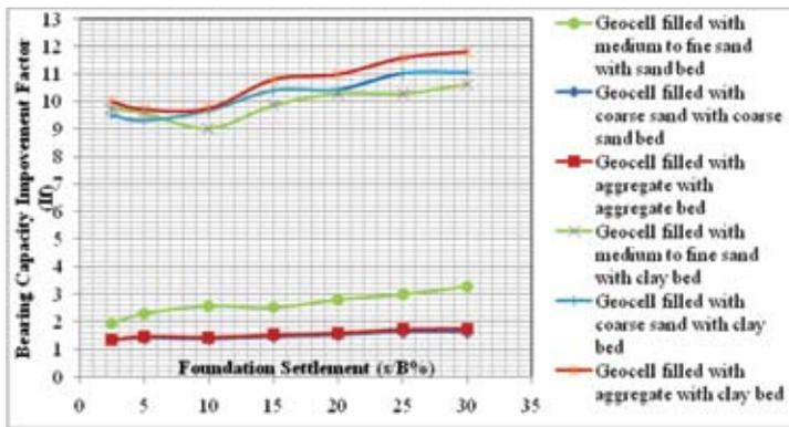
Fig. 6 : Bearing Capacity Improvement factor for Test series C
