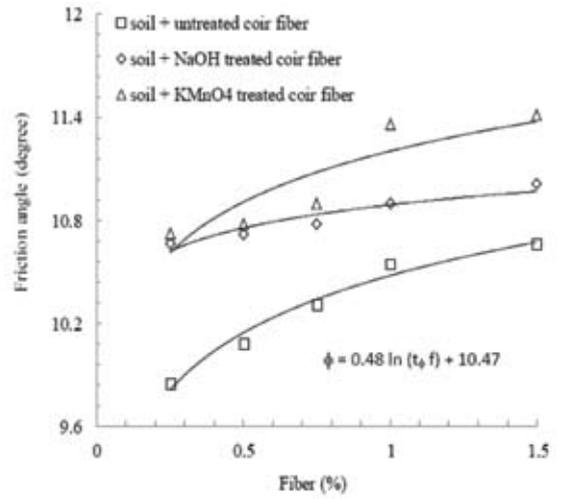
Fig. 8 : Variation friction angle with fibre content
