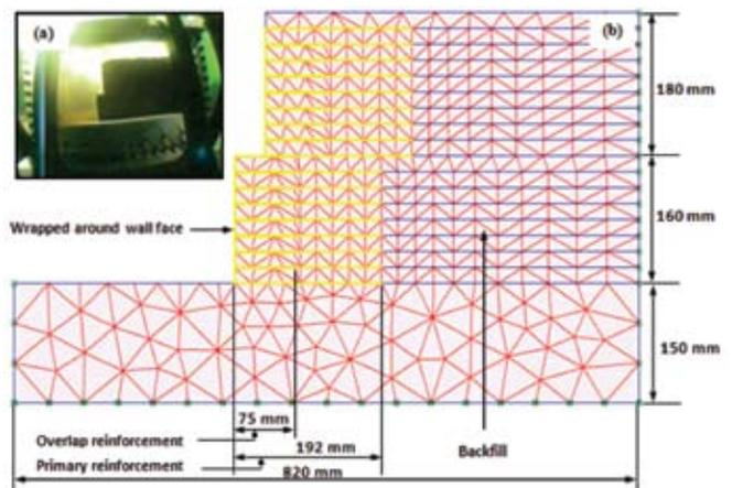
Fig. 2 : GRS two-tier wall model: (a) centrifuge at initial condition; (b) finite element setup and initial mesh
