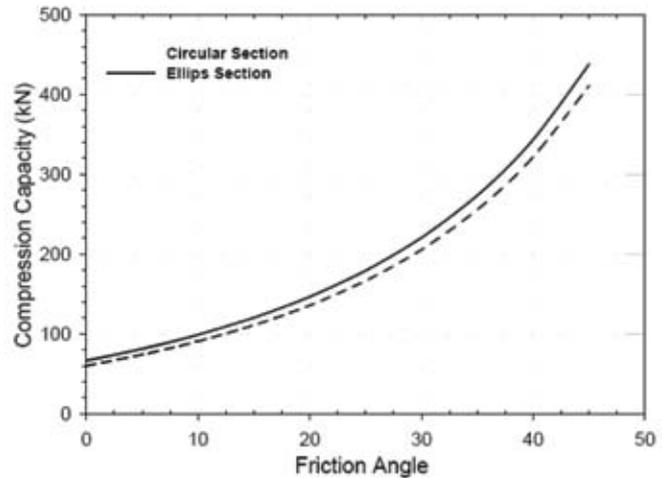
**Fig. 7 :** Variation of compression capacity with internal friction angle of soil
