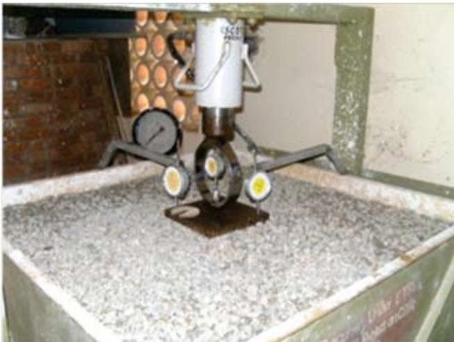
Fig. 2 : Test set up with 6 mm aggregate fill
