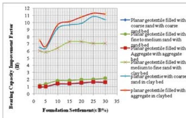
**Fig. 5** : Bearing Capacity Improvement factor for Test series B
