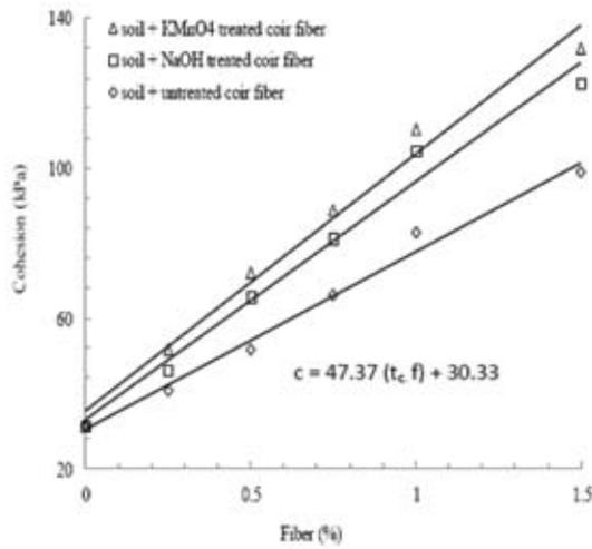
Fig. 7 : Variation cohesion with fibre content
