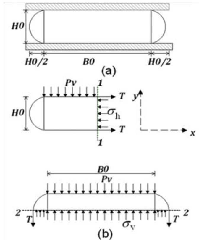
**Fig. 2 :** Geometrical form of soilbag with semi-circular boundary conditions, (b) soilbag under the pressure and tensile force T in cross-section 1 and 2.
