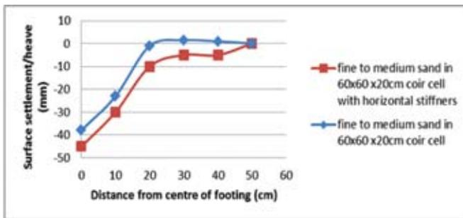
Fig. 13 : Heaving or settlement of clay surface for test series E
