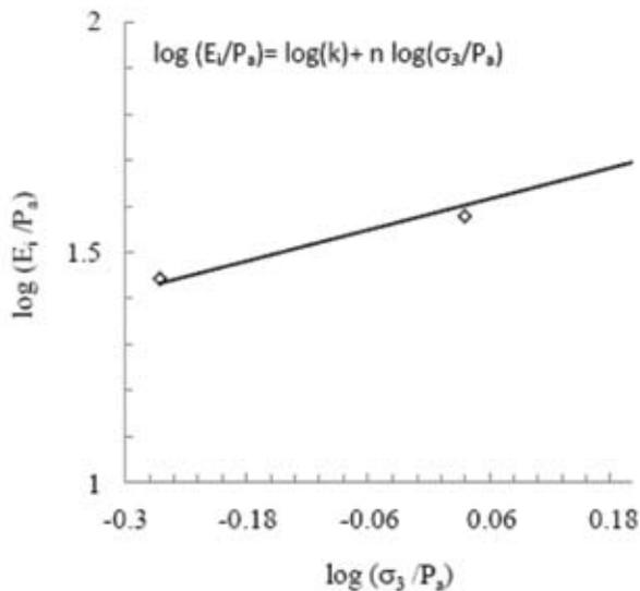
Fig. 6 : Plot for the determination of parameters k and n for soil
