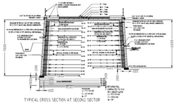
**Fig. 3:** Typical geosynthetic layout for Eluru Geosynthetic Reinforced soil Wall
