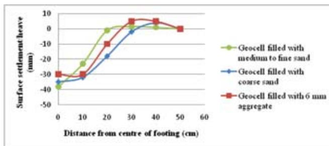
Fig. 11 : Heaving or settlement of clay surface for test series C
