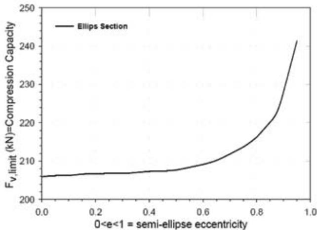
**Fig. 5 :** Changes in bearing capacity of soilbag for variable changes in eccentricity
