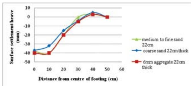
Fig. 9 : Heaving or settlement of clay surface for test series A
