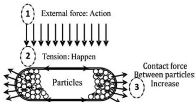
Fig. 1 : External loading process on soilbag
