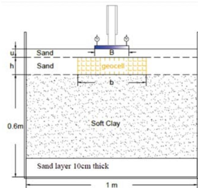
Fig. 1 : Schematic diagram of test set-up
