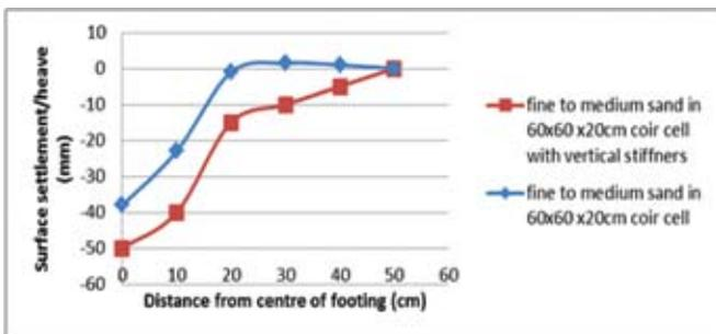
Fig. 14 : Heaving or settlement of clay surface for test series F
