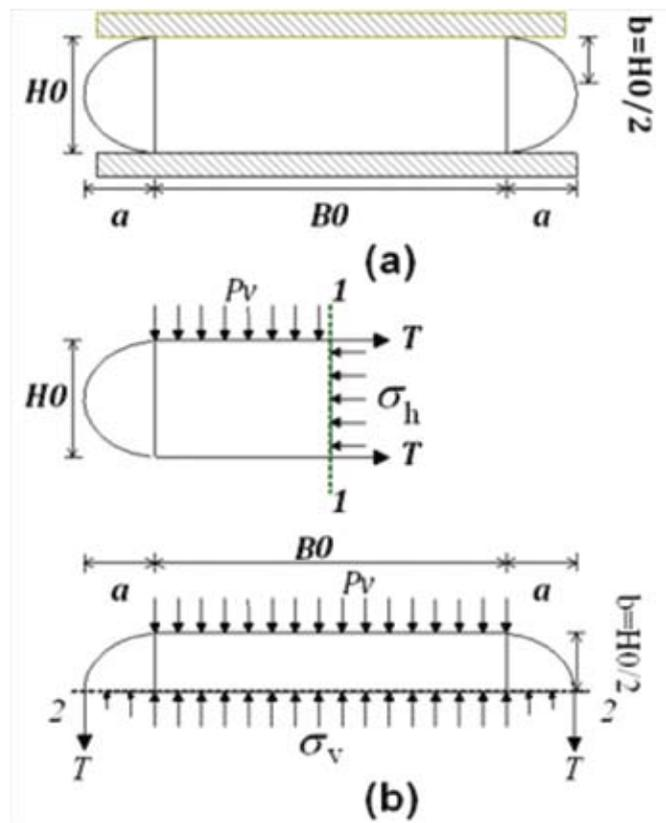
**Fig. 3 :** Geometrical form of soilbag with semi-elliptical boundary conditions, (b) soilbag under the pressure  $p_v$  and tensile force  $T$  in cross-section 1 and 2.
