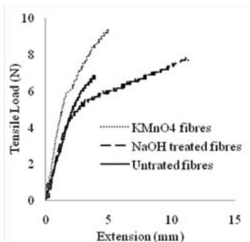
**Fig. 2 :** Tensile load extension curve for the untreated and treated coir fibre
