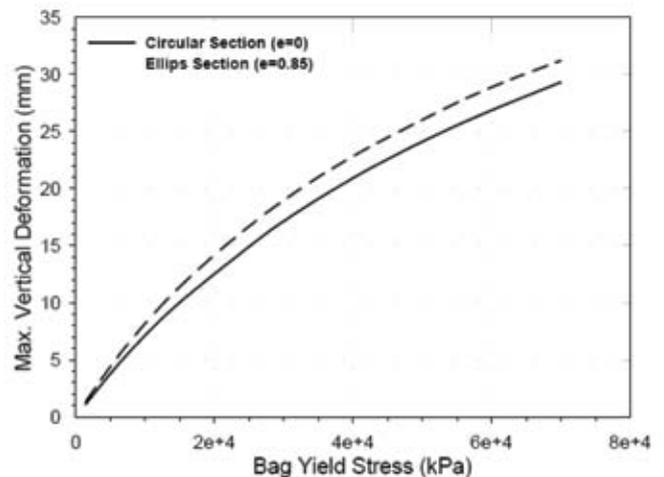
**Fig. 8 :** Maximum vertical deformation of soilbag under vertical compression
