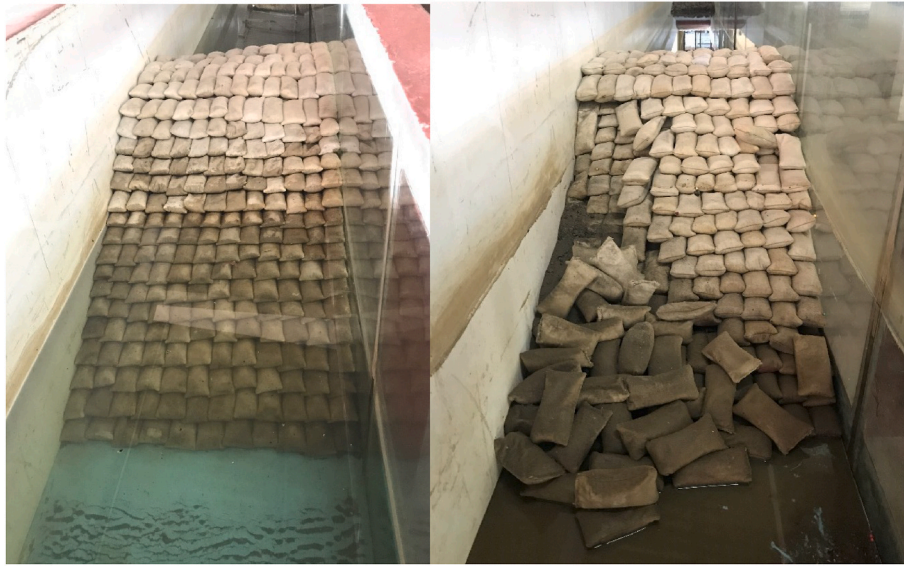
Fig. 4. Bag 1 Double layer configuration, (a.) Stable (DC0) after exposure of 0.06 m wave heights, (b.) Total Failure (DC4) after exposure to 0.16 m wave heights.
