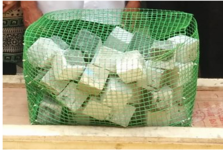
Fig. 3. Prepared Specimens filled in Gabion.
