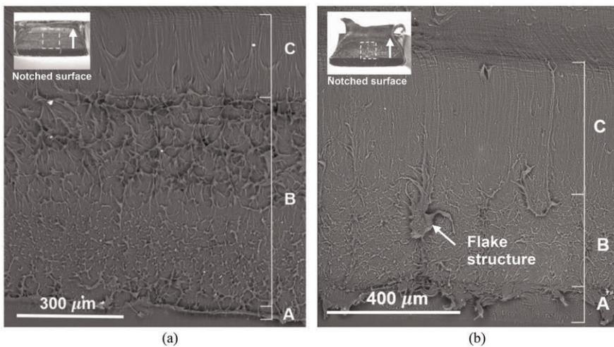
Figure 2. SEM micrographs of the fracture surface from: (a) a HDPE specimen aged for 6.8 years ( $SCR_{7\text{years}} = 5$  h;  $SCR_{7\text{years}}/SCR_0 < 0.01$ ); and (b) a LLDPE specimen aged for 4 years ( $SCR_{4\text{years}} = 617$  h;  $SCR_{4\text{years}}/SCR_0 = 0.03$ ).
