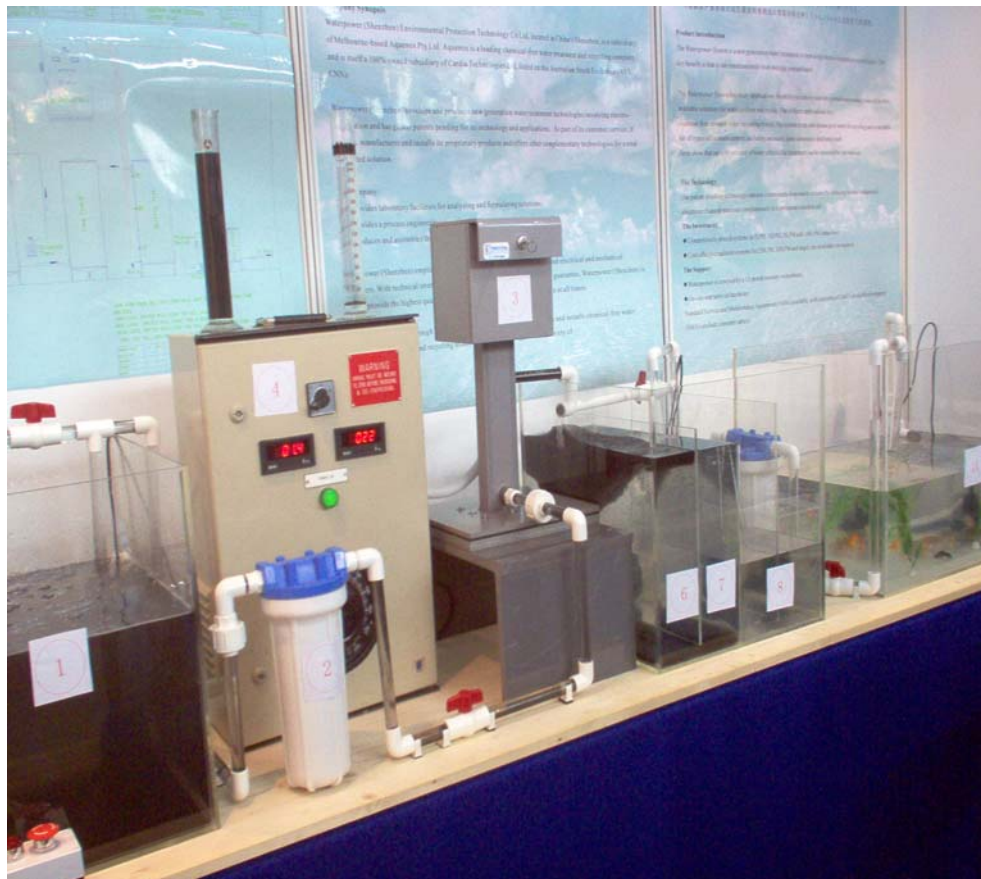
Above image shows “live” demonstration of the effectiveness of the Aquenox Waterpower process. This example shows dye effluent (collected in tank at left) treated through the Waterpower process, resulting in clean water discharged into fish-tank (shown at right).
