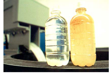
Sample obtained directly from a Waterpower cell (bottle-left) shows high separation efficiency on a multiple component sample (bottle-right).
