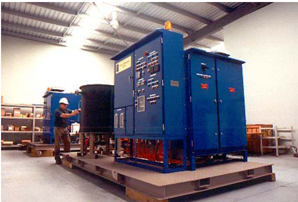
An integrated control system maintains all run parameters, valve conditions and includes safety interlocks for completely unattended operations.
