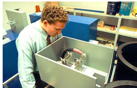
Low cost locally available electrode plates are easily removed and replaced on a periodic basis.
