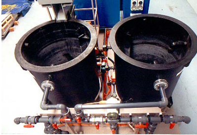
Each system includes sophisticated valving that operates automatically for incoming sample feed, level compliance, discharge to a development tank and outlet.
