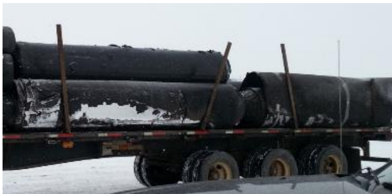
Figure 2.1: Packaging of a drainage geocomposite damaged before arrival onsite, making the product impossible to install (photo courtesy Scorpion Containment).
