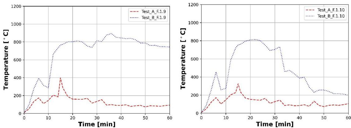
Figure 6. Temperature on the 1<sup>st</sup> floor of the main wall: (left) F.1.9, (right) F.1.10.
