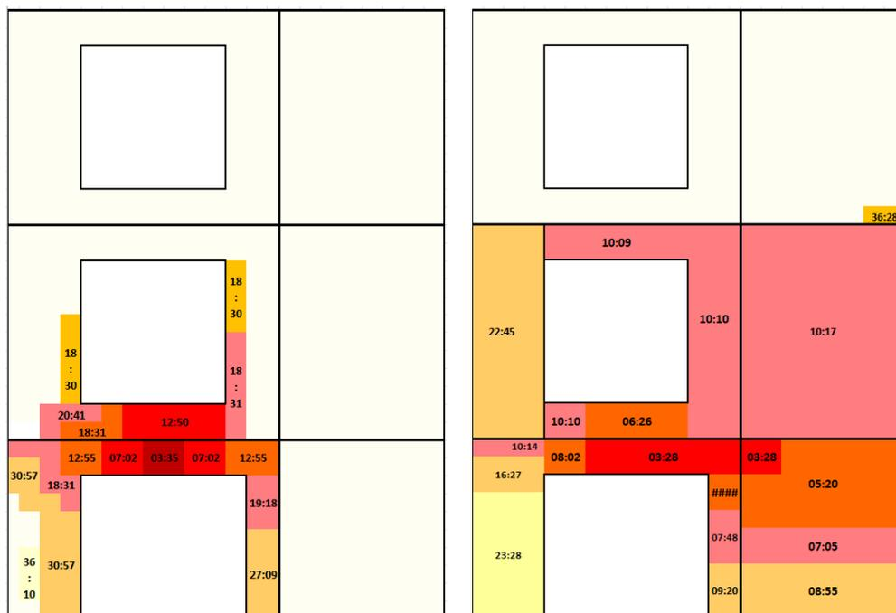
Figure 8. Flame spread comparison between Test A (left) and Test B (right).
