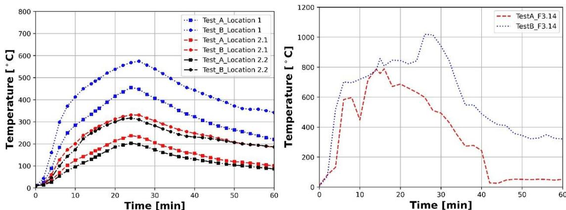
Figure 4. (left) Plate thermometer temperature outside the chamber at locations 1, 2.1 and 2.2, and (left) temperature right above the chamber on the main wall.
