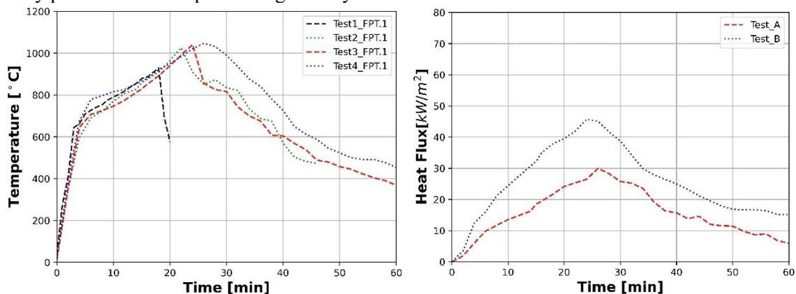
Figure 3. (left) Temperatures inside the combustion chamber in four tests and (right) heat flux at 3 m away from the facade and 1.4 m above the ground level.
