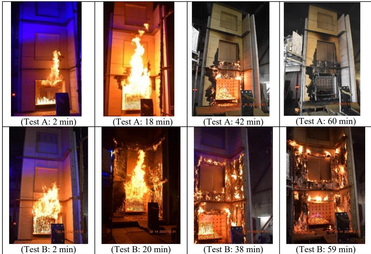
Figure 2. Snapshots captured at different times during the tests (both tests concluded after 60 mins).
