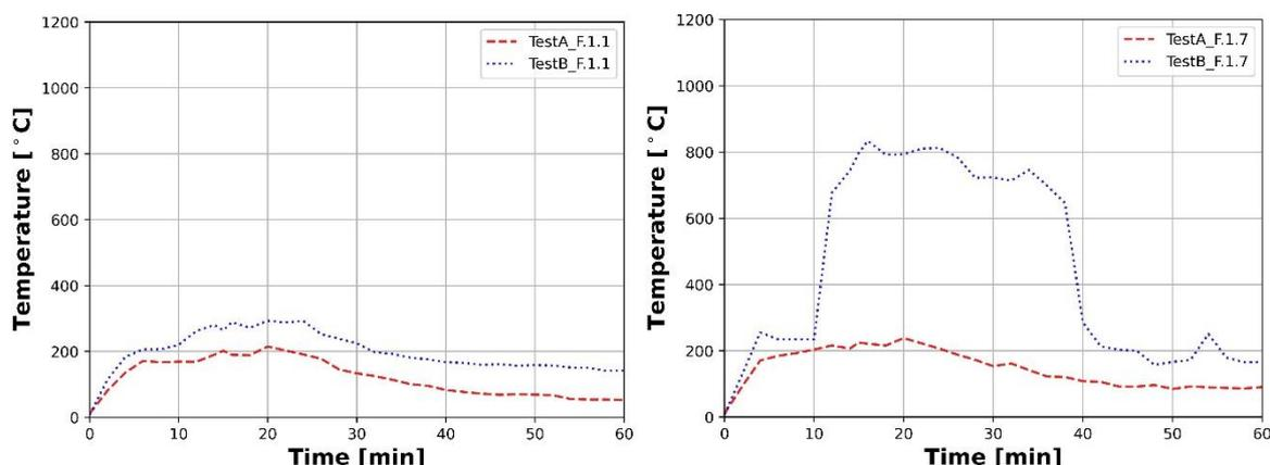
Figure 5. Temperature on the 2<sup>nd</sup> floor (left: F.1.1) and the 1<sup>st</sup> floor of the main wall (right: F.1.7).
