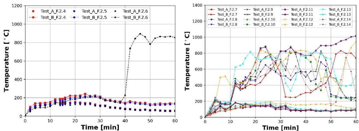
Figure 7. Vertical temperatures on the side wing: (left) 2<sup>nd</sup> floor, (right) 1<sup>st</sup> floor and ground floor.
