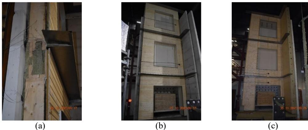
Figure 1. Build-up of the façade system (a) and the experimental set-up of Test A (b) and Test B (c).
